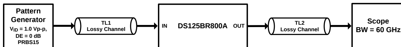
Figure 23. Test Setup Connections Diagram
