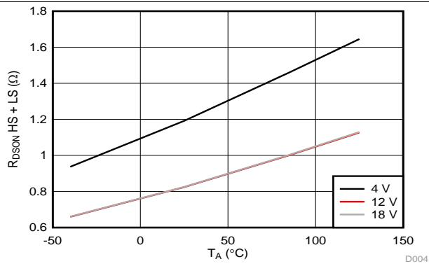
Figure 5.  $R_{DSON}$  vs Temperature
