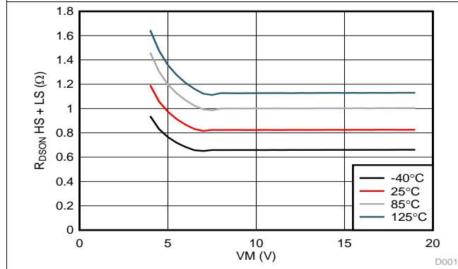
Figure 4.  $R_{DSON}$  vs  $V_M$
