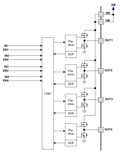
Figure 2. Motor Control Circuitry
