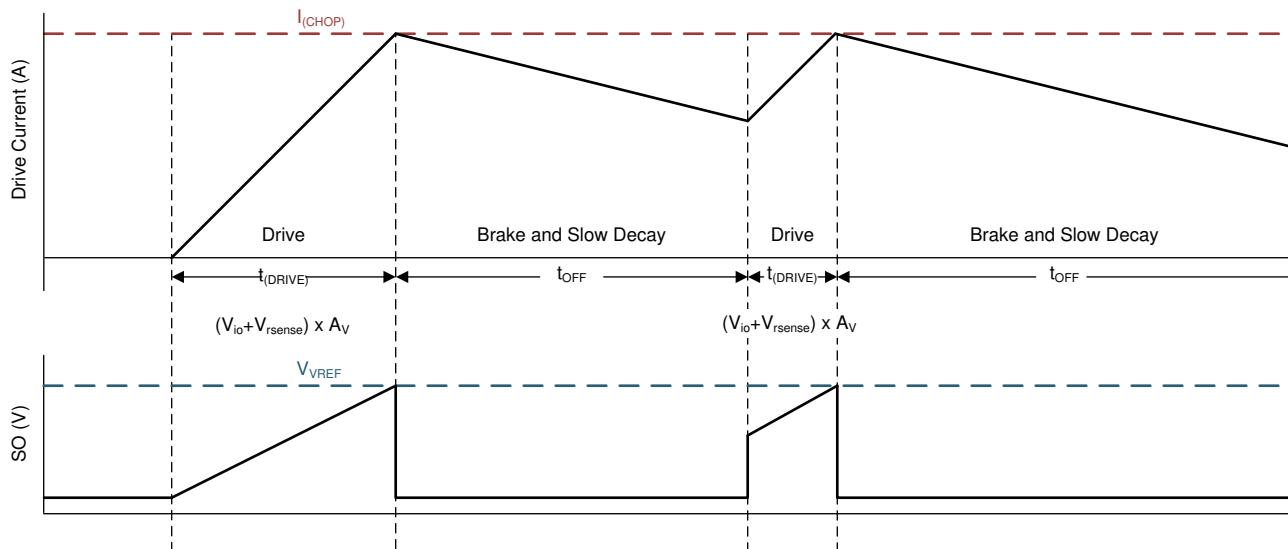
图 7-7. Current Sense Amplifier and Current Chopping Operation
