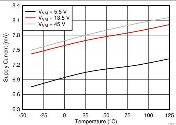
图 6-2. Supply Current vs Temperature
