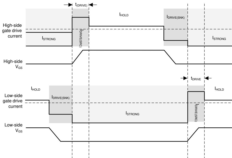
图 7-10. Gate Driver Output to Control External FETs
