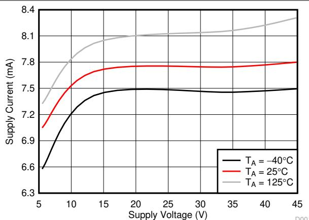
图 6-1. Supply Current vs Supply Voltage (VM)
