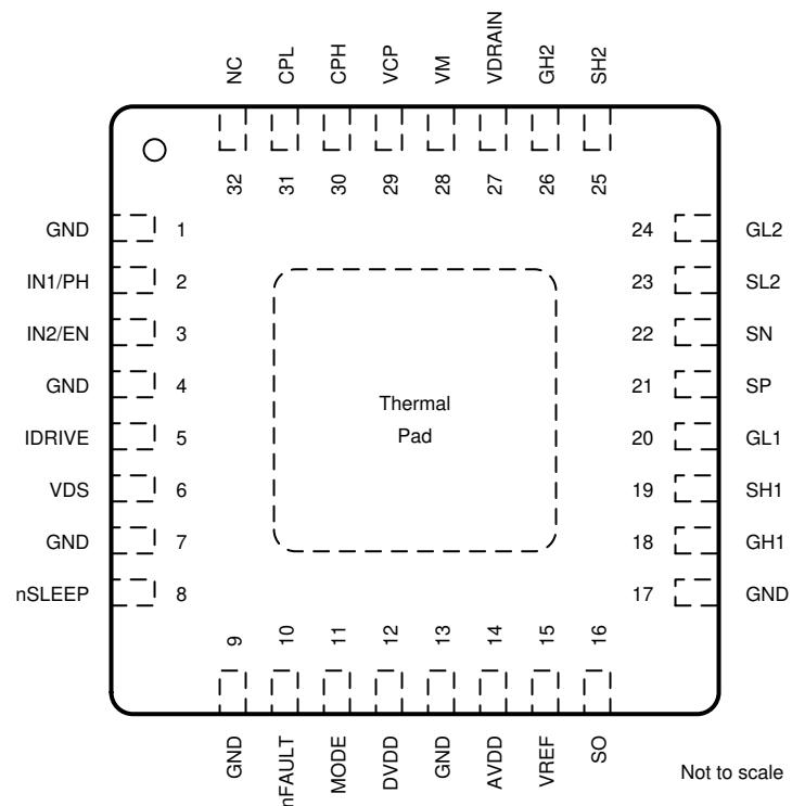
图 5-1. DRV8702-Q1 RHB Package With Wettable Flanks 32-Pin VQFN Top View
