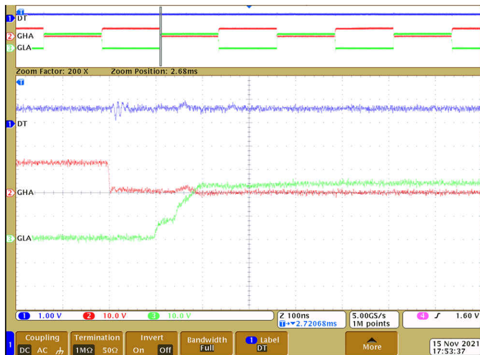
图 9-16. Driver dead time of 100 ns (DT = 10 k \Omega to GND)
