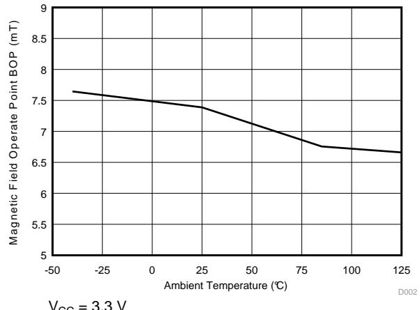
Figure 4. DRV5033AJ,  $B_{OP}$  vs Temperature
