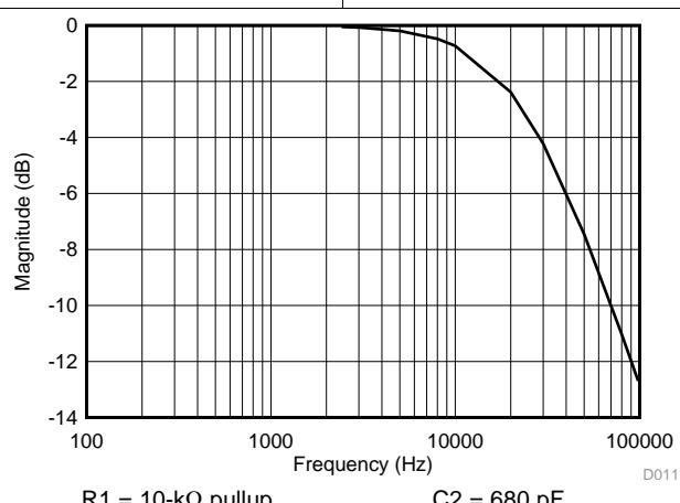
**Figure 21. Low-Pass Filtering**
