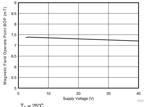
Figure 3. DRV5033AJ,  $B_{OP}$  vs  $V_{CC}$
