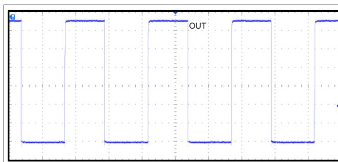
**Figure 19. 10-kHz Switching Magnetic Field**
