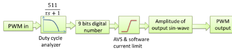
Figure 4. PWM Command Input Controls the Output Peak Amplitude
