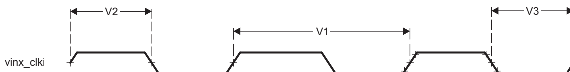
图 5-20. Video Input Ports Clock Signal
