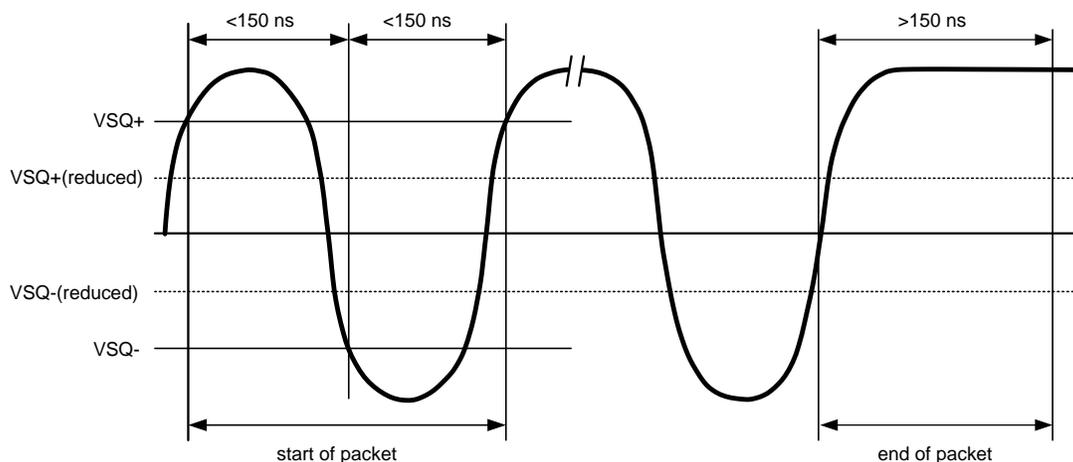
**Figure 7-5. 10BASE-T Twisted Pair Smart Squelch Operation**
