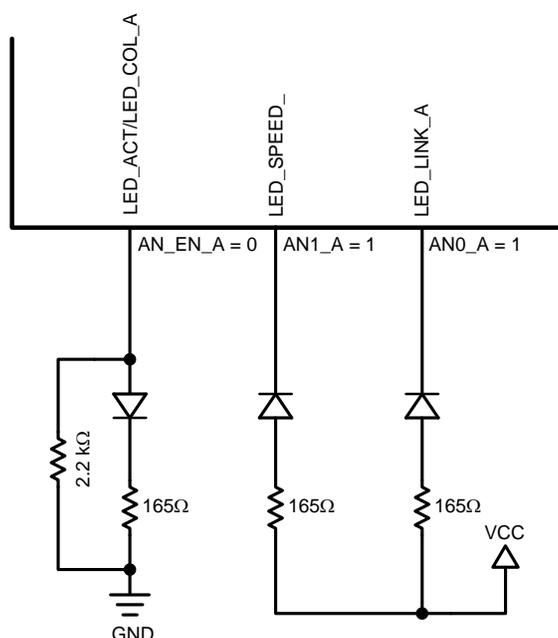
**Figure 5-2. AN Strapping and LED Loading Example**
