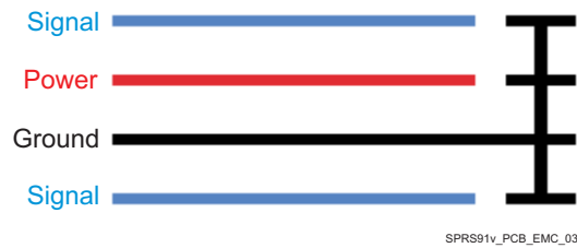
图 7-13. Guard Ring Routing
