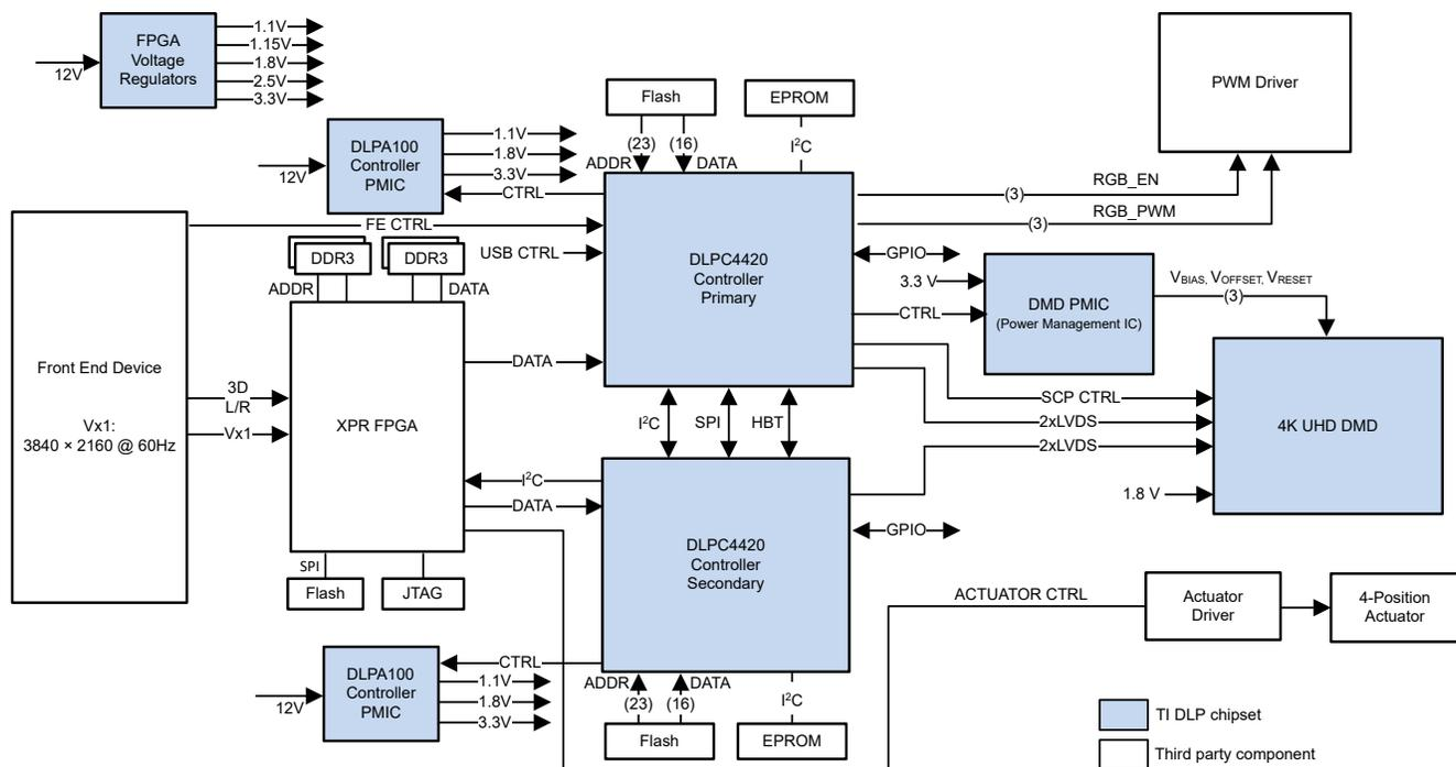
图 8-1. Typical 4K UHD LED Display Application
