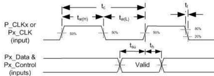
图 6-6. Port1, Port2, and Port3 Input Interface
