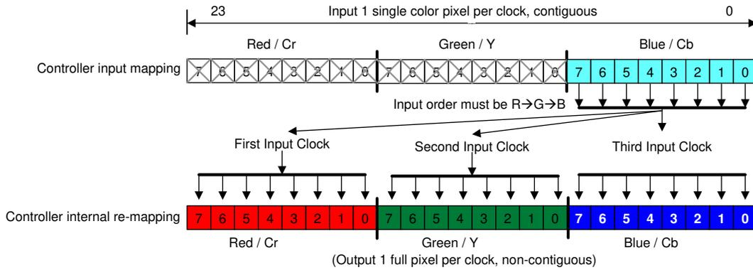
**图 7-6. 8-Bit RGB-888 or YCbCr-888 I/O Mapping**
