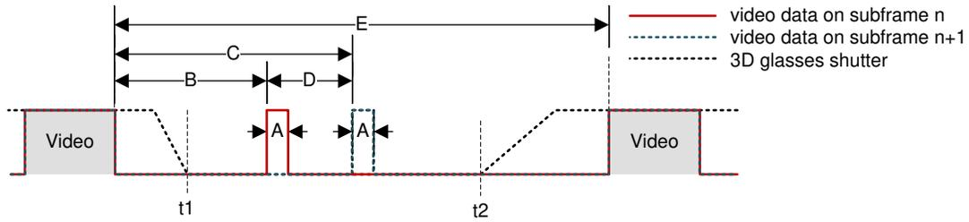
The time offset of DLP Link pulses at the end of a subframe alternates between B and B+D where D is the delta offset.
