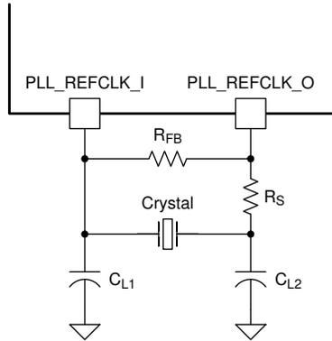
$C_L$  = Crystal load capacitance (farads)
