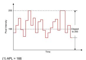
图 7-10. Source Pixels for a Color Channel
