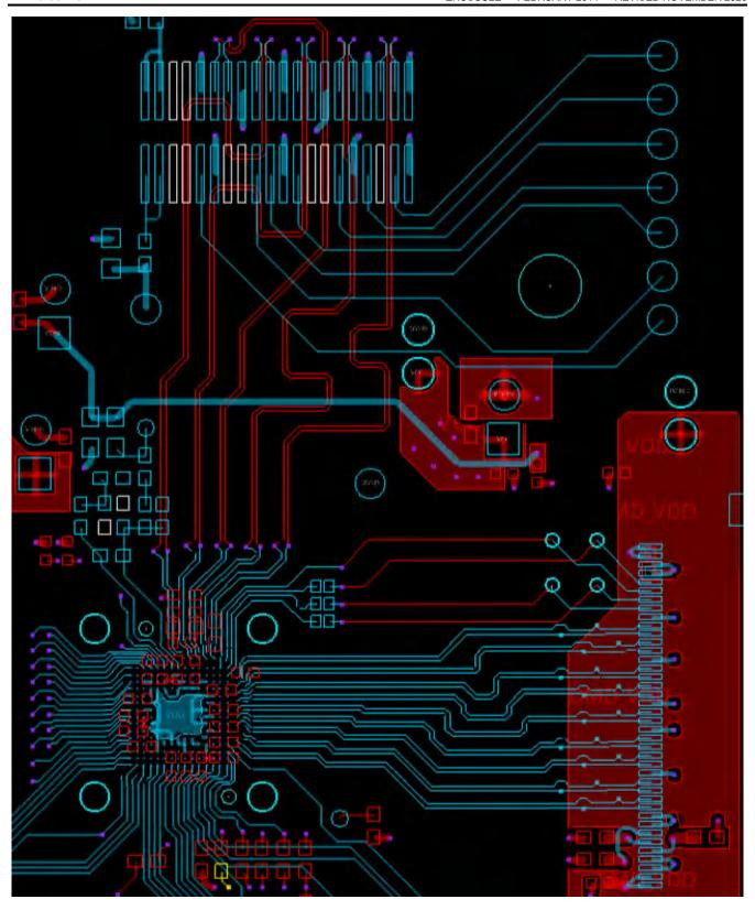
图 10-4. Layout Recommendation with DSI (DLPC3433 only)
