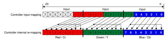
图 7-3. RGB-666 and YCbCr-666 I/O Mapping
