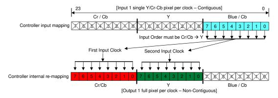
图 7-7. 8-Bit Serial YCbCr-422 I/O Mapping
