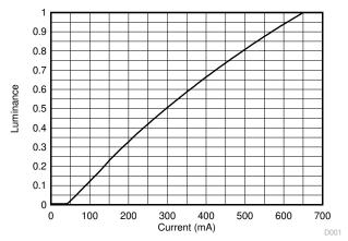
图 8-3. Typical Luminance vs Current
