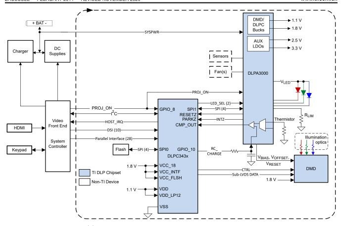
图 8-2. Typical Application Diagram (using DLPA3000)
