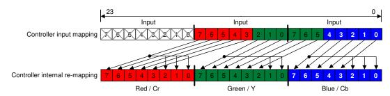
图 7-4. RGB-565 and YCbCr-565 I/O Mapping
