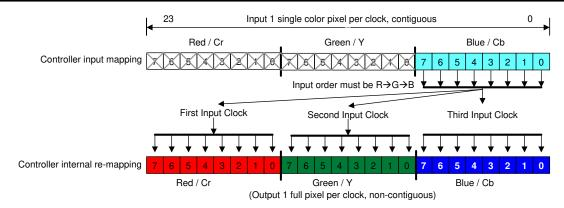
图 7-6. 8-Bit RGB-888 or YCbCr-888 I/O Mapping
