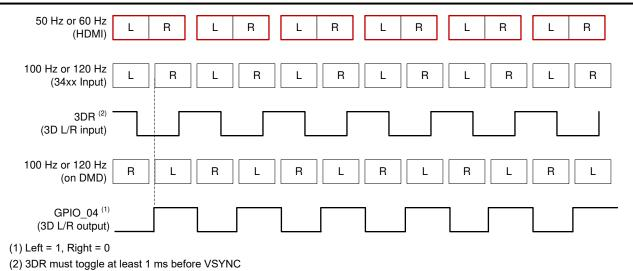
图 7-1. 3D Display Left and Right Frame Timing
