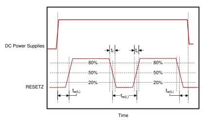
图 6-6. Power-Up and Power-Down RESETZ Timing
