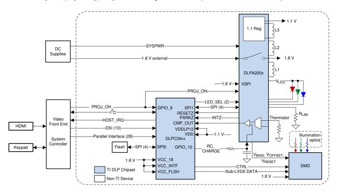
图 8-1. Typical Application Diagram (using DLPA200x)
