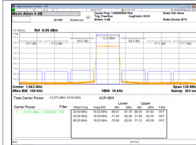
图 8-4. Dual band ACPR Performance in Downlink Band 3 with On-chip PLL
