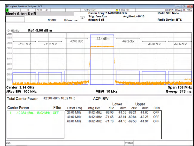
图 8-5. Dual band ACPR Performance in Downlink Band 1 with On-chip PLL
