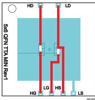
Max  $R_{\theta JA} = 50^\circ\text{C}/\text{W}$
