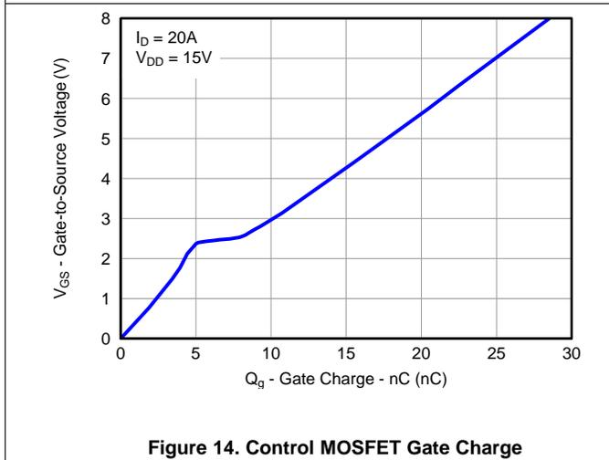
Figure 14. Control MOSFET Gate Charge
