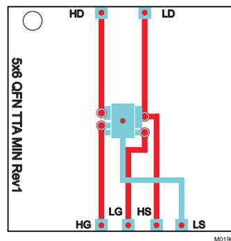
Max  $R_{\theta JA} = 102^\circ\text{C}/\text{W}$
