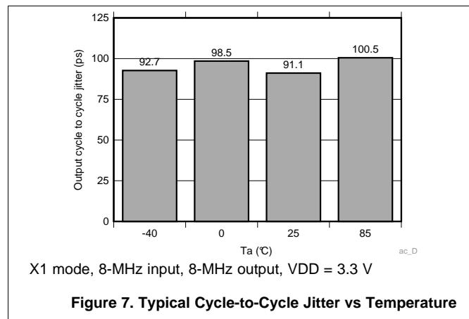
Figure 7. Typical Cycle-to-Cycle Jitter vs Temperature
