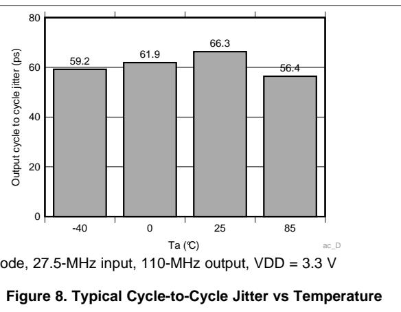
Figure 8. Typical Cycle-to-Cycle Jitter vs Temperature
