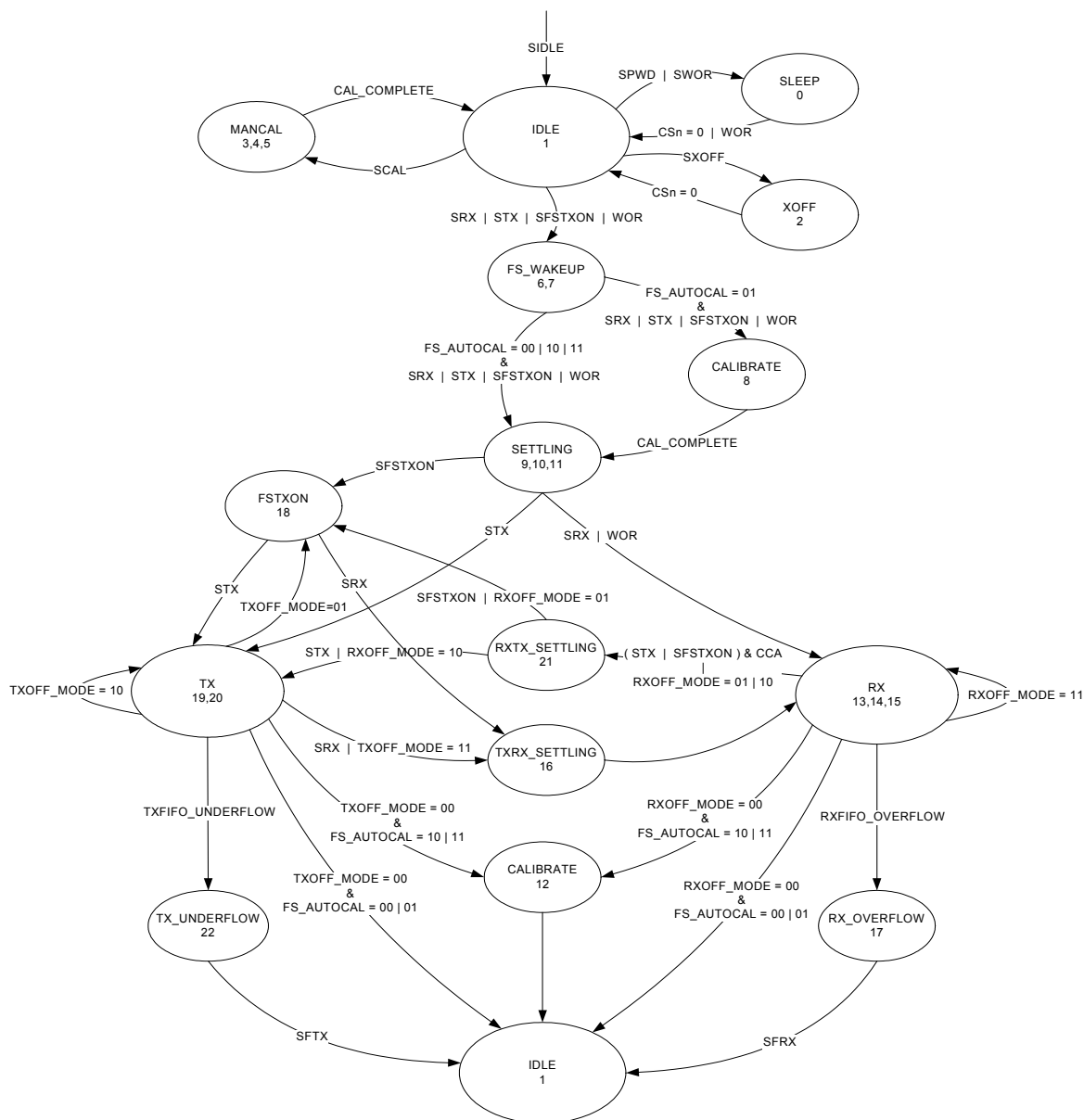
Figure 16: Complete Radio Control State Diagram
