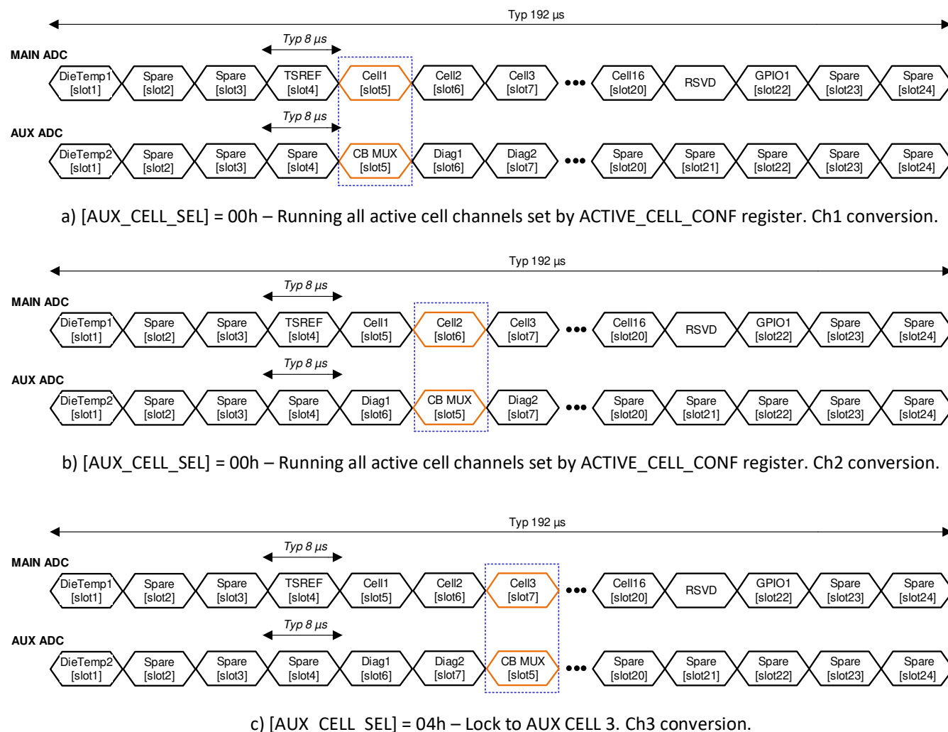
图 8-11. Synchronization between MAIN and AUX ADC Sampling
