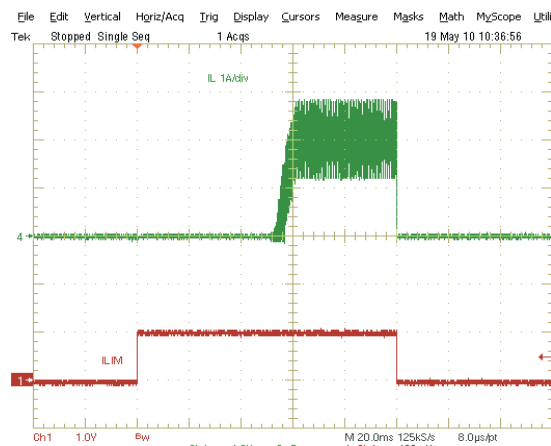
CH1: ILIM, 1V/div, CH4: inductor current, 1A/div, 20ms/div
