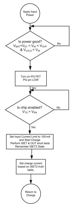
图 8-3. BQ2404x Power-Up Flow Diagram
