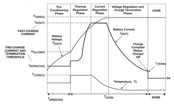
图 8-1. Charging Profile With Thermal Regulation
