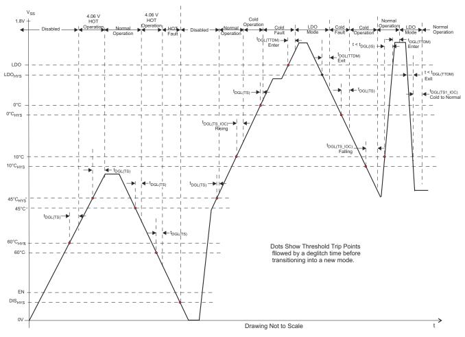
图 8-2. TS Battery Temperature Bias Threshold and Deglitch Timers
