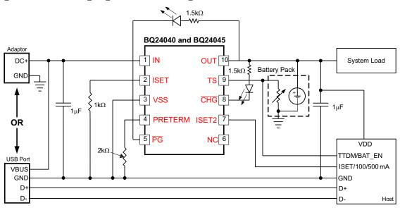
图 9-1. Typical Application Circuit: BQ24040 and BQ24045
