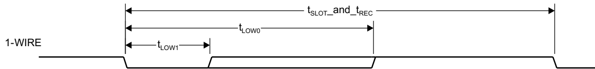
图 5-109. 1-Wire Write Bit Timing (Command/Address or Data)
