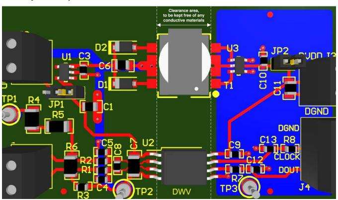
Figure 55. Recommended Layout of the AMC1336-Q1
