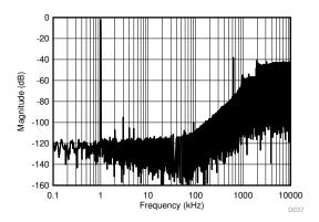
$sinc^3$  filter, OSR = 1,  $f_{CLKIN}$  = 20 MHz,  $f_{IN}$  = 1 kHz
