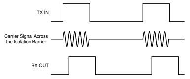
Figure 44. OOK-Based Modulation Scheme
