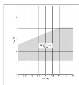
Figure 40. Common-Mode Input Voltage Range With a Clipping Differential Input Signal of ±1.25 V
