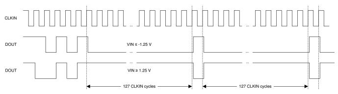
Figure 48. Out-of-Range Output of the AMC1336-Q1
