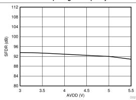
Figure 29. Spurious-Free Dynamic Range vs High-Side Supply Voltage
