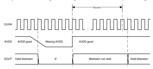
Figure 49. Fail-Safe Output of the AMC1336-Q1
