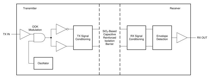
Figure 43. Block Diagram of an Isolation Channel
