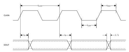
Figure 1. Digital Interface Timing
