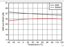
Figure 20. Signal-to-Noise Ratio and Signal-to-Noise + Distortion vs Temperature
