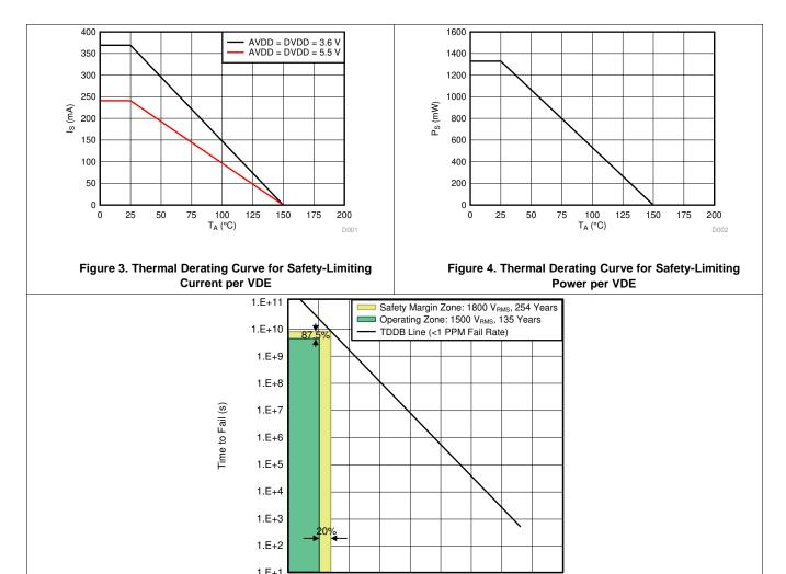
$T_A$  up to 150°C, stress-voltage frequency = 60 Hz, isolation working voltage = 1500  $V_{RMS},$  operating lifetime = 135 years
