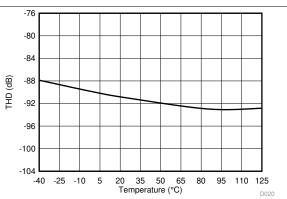
Figure 25. Total Harmonic Distortion vs Temperature
