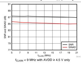
Figure 21. Signal-to-Noise Ratio and Signal-to-Noise +
