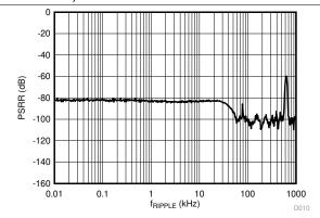
Figure 18. Power-Supply Rejection Ratio vs Ripple Frequency
