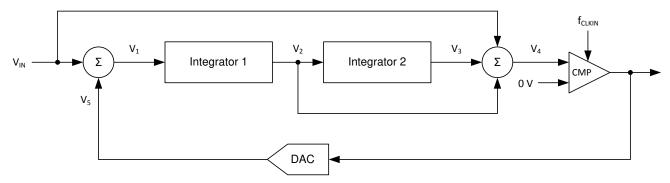
Figure 42. Block Diagram of a Second-Order Modulator
