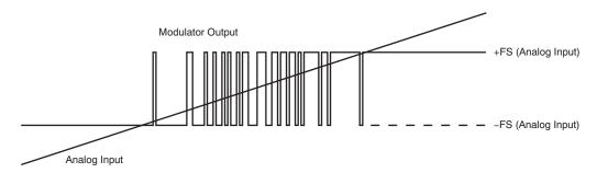
Figure 45. Analog Input versus the AMC1336-Q1 Modulator Output
