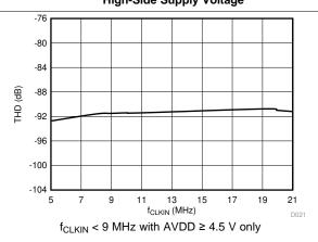
Figure 26. Total Harmonic Distortion vs Clock Frequency
