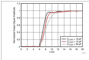
Figure 46. DOUT Rising Edge With Different Capacitive Loads
