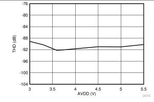
Figure 24. Total Harmonic Distortion vs High-Side Supply Voltage
