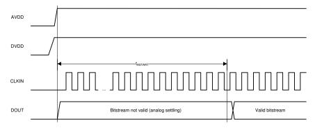
Figure 2. Device Start-Up Timing
