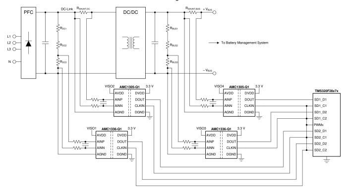
Figure 51. The in an On-Board Charger Application
