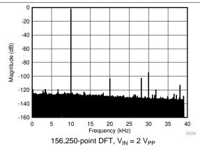
Figure 35. Frequency Spectrum with 10-kHz Input Signal
