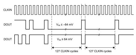
图 7-5. Output of the AMC1306M05-Q1 in Case of an Input Overrange
