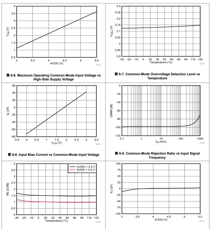
图 6-10. Integral Nonlinearity vs Temperature
