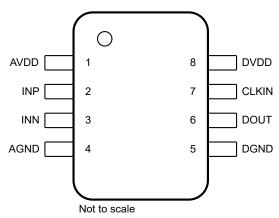
图 5-1. DWV Package, 8-Pin SOIC (Top View)
