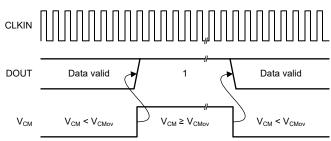
图 7-6. Output of the AMC1306M05-Q1 in Case of a Common-Mode Overvoltage
