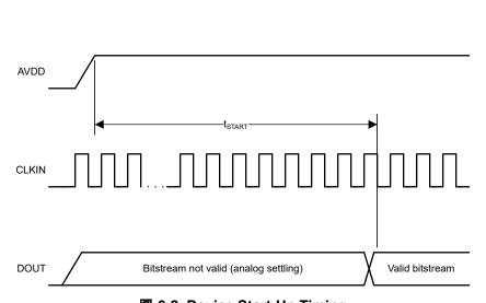
图 6-2. Device Start-Up Timing
