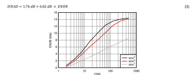
图 8-3. Measured Effective Number of Bits vs Oversampling Ratio
