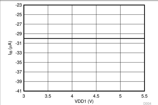
图 6-14. Input Bias Current vs High-Side Supply Voltage
