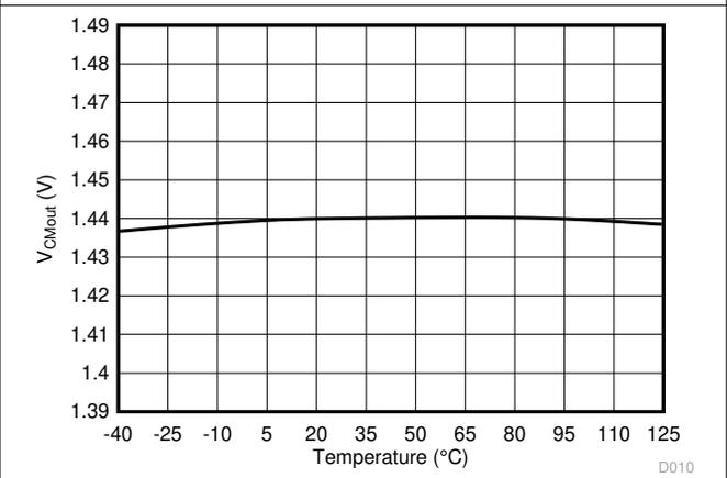
图 6-34. Output Common-Mode Voltage vs Temperature
