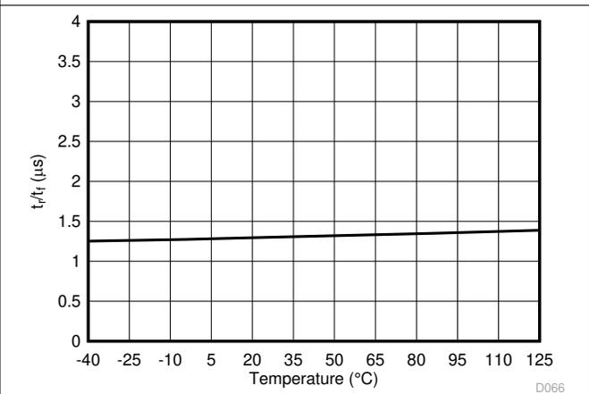
图 6-40. Output Rise and Fall Time vs Temperature
