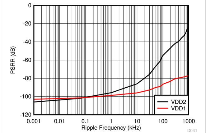
图 6-32. Power-Supply Rejection Ratio vs Ripple Frequency
