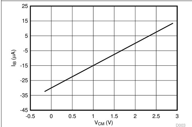
图 6-13. Input Bias Current vs Common-Mode Input Voltage
