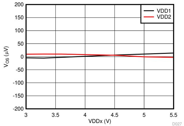
图 6-8. Input Offset Voltage vs Supply Voltage
