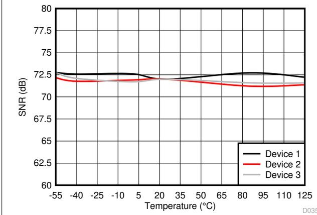
图 6-31. Signal-to-Noise Ratio vs Temperature
