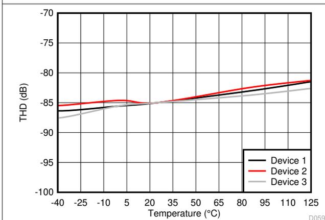
图 6-27. Total Harmonic Distortion vs Temperature
