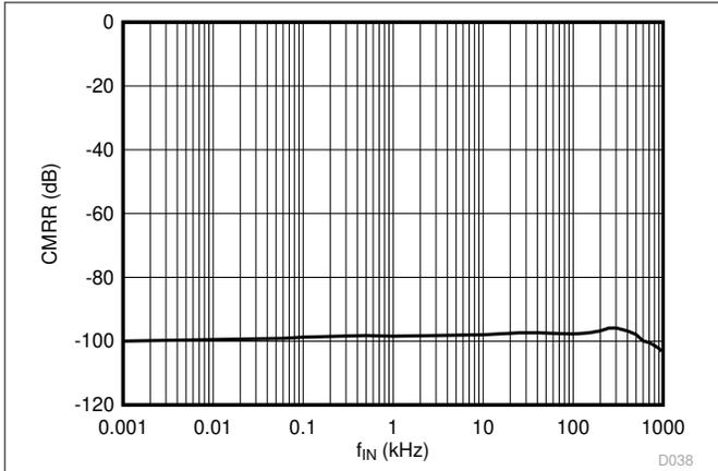
图 6-11. Common-Mode Rejection Ratio vs Input Frequency
