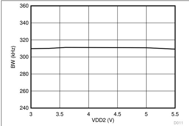
图 6-35. Output Bandwidth vs Low-Side Supply Voltage
