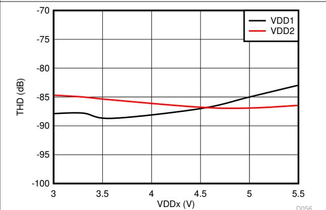
图 6-26. Total Harmonic Distortion vs Supply Voltage
