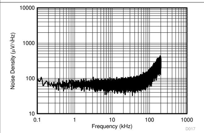
图 6-28. Input-Referred Noise Density vs Frequency
