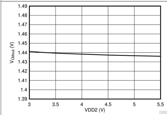
图 6-33. Output Common-Mode Voltage vs Low-Side Supply Voltage
