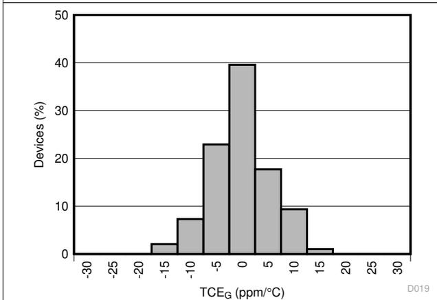
图 6-19. Gain Error Drift Histogram
