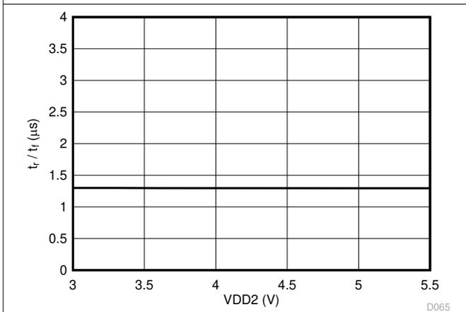
图 6-39. Output Rise and Fall Time vs Low-Side Supply
