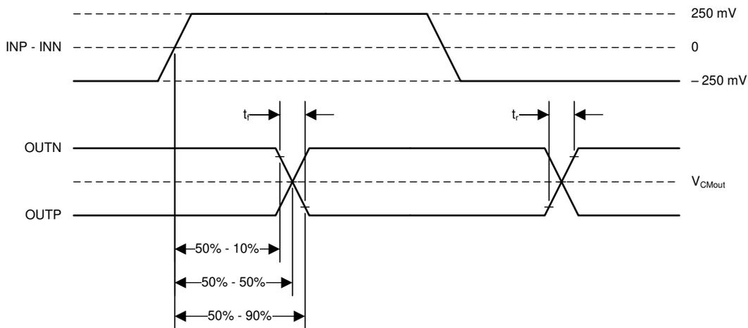
**图 6-1. Rise, Fall, and Delay Time Definition**
