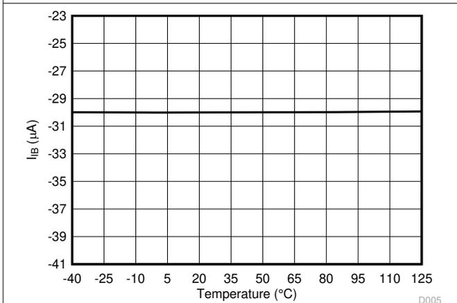
图 6-15. Input Bias Current vs Temperature
