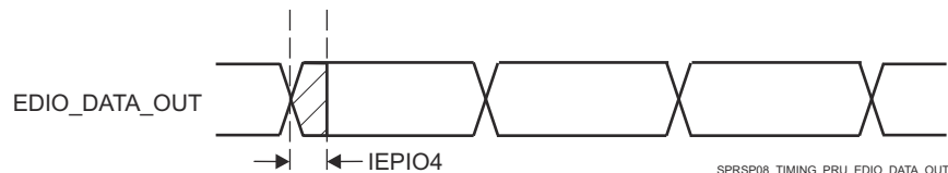
图 6-106. PRU_ICSSG PRU IEP Digital IOs Timing
