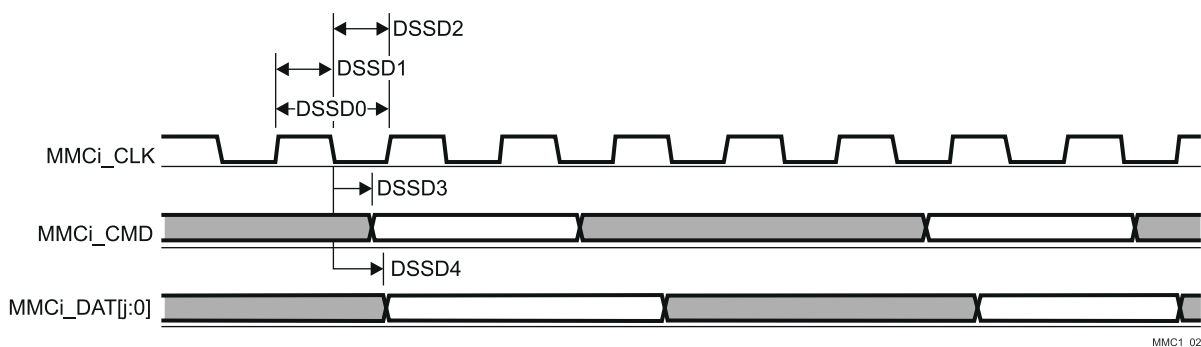
图 6-73. eMMC/SD/SDIO in - Default Speed - Transmitter Mode
