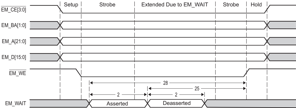
图 10-54. EMIF16 \text{EM\_WAIT} Write Timing Diagram
