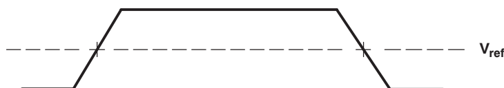
Figure 6-2. Input and Output Voltage Reference Levels for AC Timing Measurements
