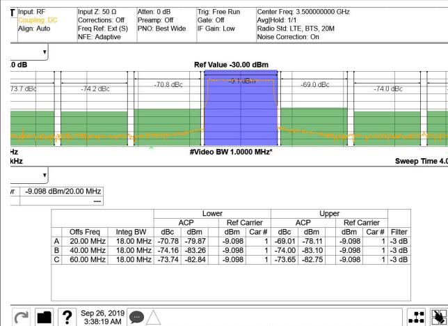
图 5-449. TX 20-MHz LTE Output Spectrum at 3.5 GHz (Band 42)
