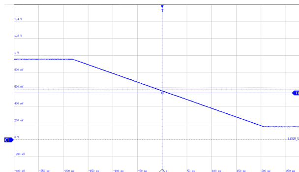
24 mA (0xF45D) to 4 mA (0x0BA3) measured on 40- \Omega shunt
