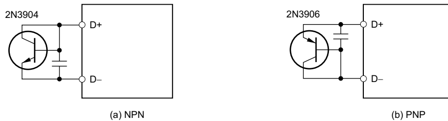
图 7-6. Remote Temperature Sensor Using Transistor
