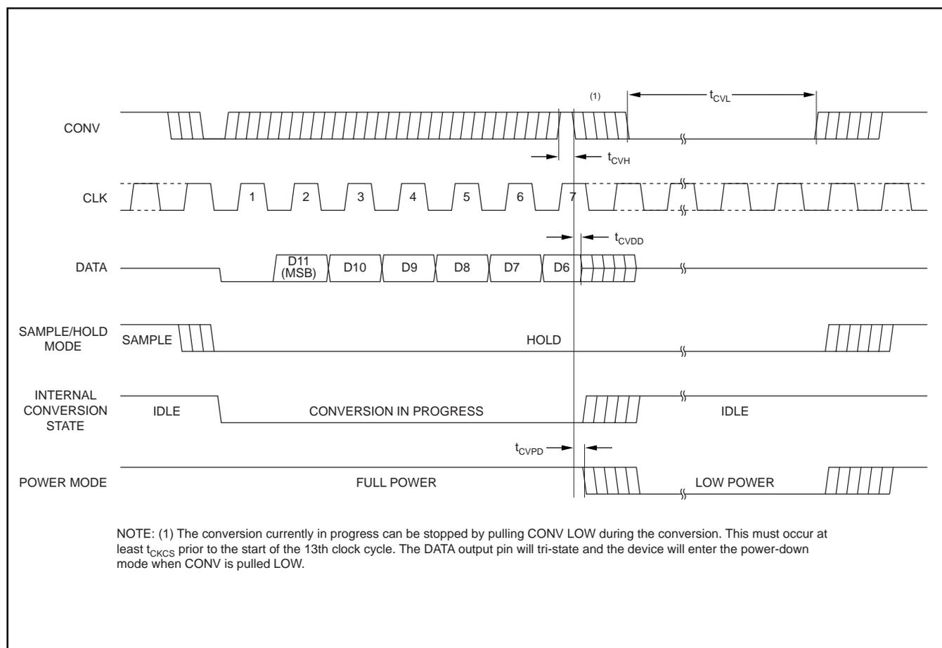
FIGURE 6. Short-cycle Timing.
