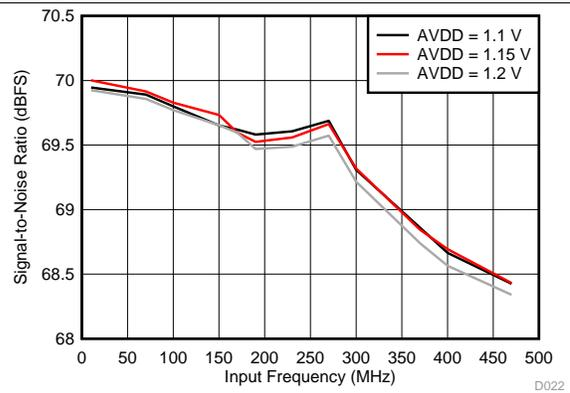
图 23. SNR vs Input Frequency and AVDD Supply
