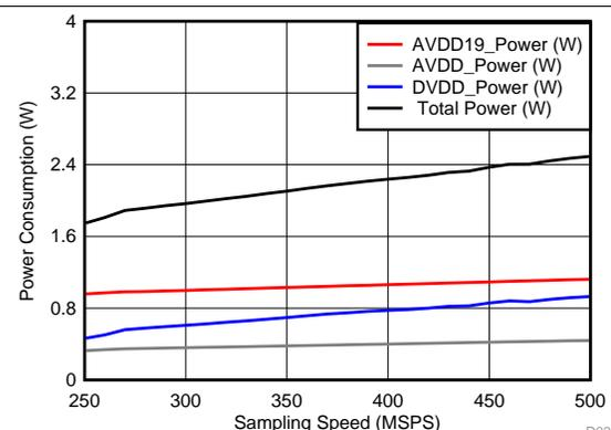
图 35. Power Consumption vs Sampling Speed
