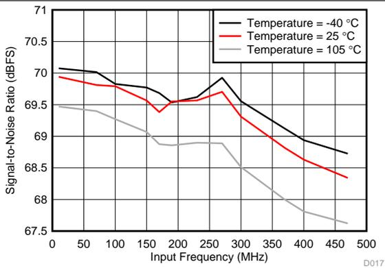
图 18. SNR vs Input Frequency and Temperature
