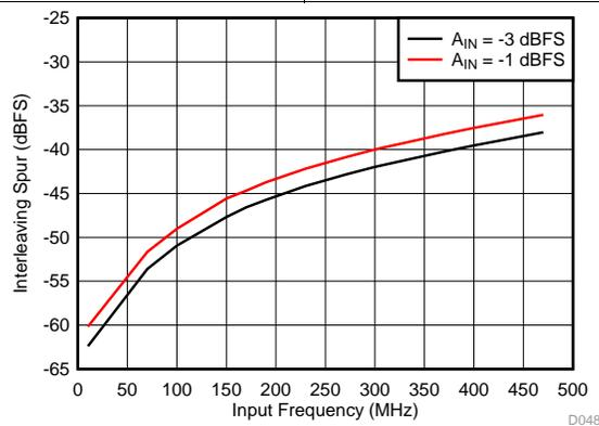
图 45. Interleaving Spur vs Input Frequency
