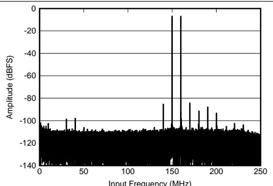
$f_{\text{IN1}} = 340\text{ MHz}$ ,  $f_{\text{IN2}} = 350\text{ MHz}$ ,  $\text{IMD} = 84.34\text{ dBFS}$ ,
