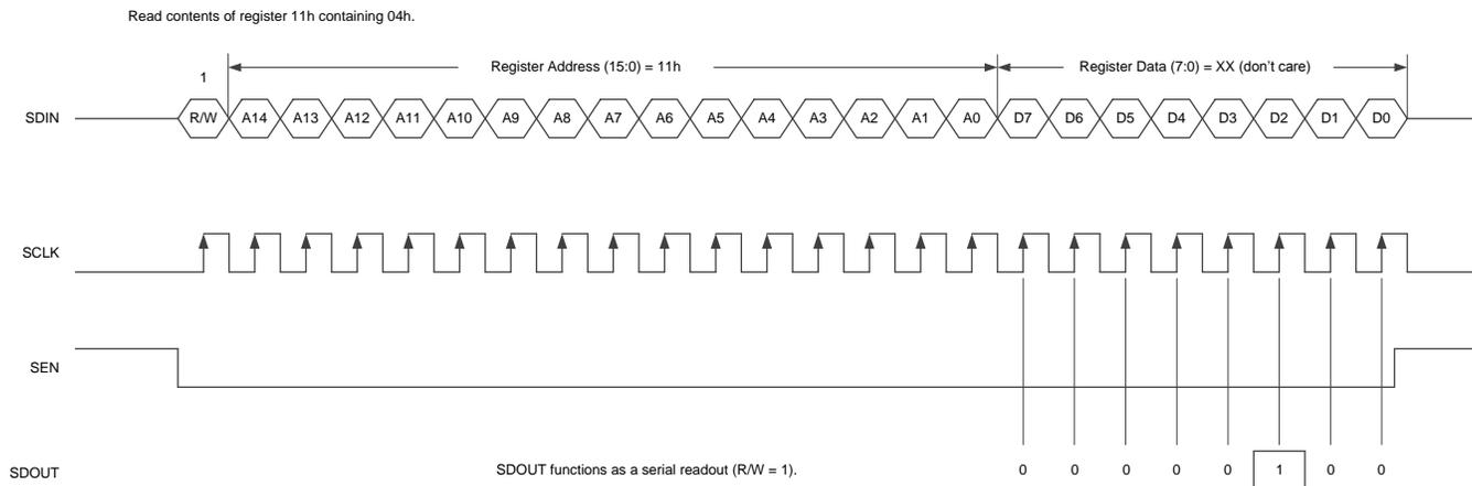
图 75. Serial Interface 4-Wire Read Timing Diagram
