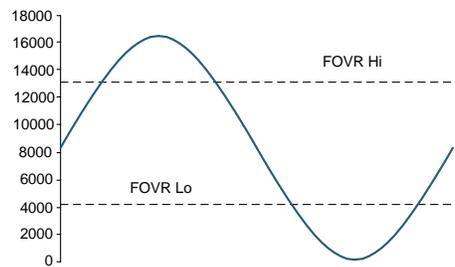
**图 64. FOVR High and FOVR Low Thresholds**
