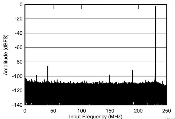
$f_{\text{IN}} = 270\text{ MHz}$ ,  $A_{\text{IN}} = -3\text{ dBFS}$ ,  $\text{SNR} = 69.27\text{ dBFS}$ ,
