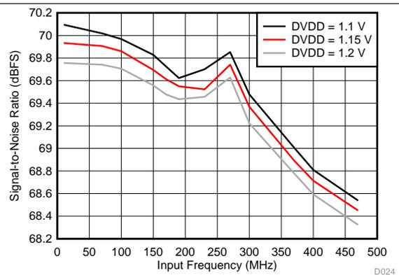
图 25. SNR vs Input Frequency and DVDD Supply
