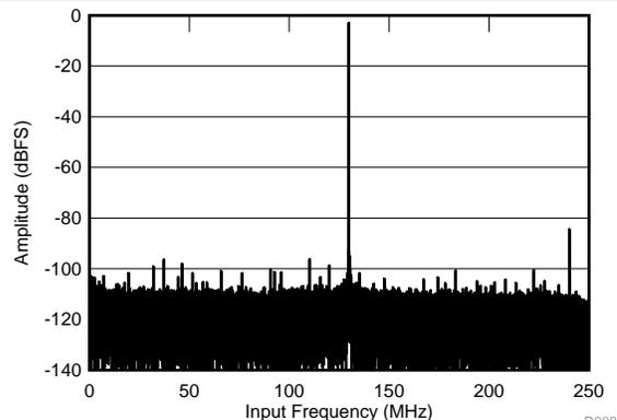
$f_{\text{IN}} = 370\text{ MHz}$ ,  $A_{\text{IN}} = -3\text{ dBFS}$ ,  $\text{SNR} = 68.36\text{ dBFS}$ ,
