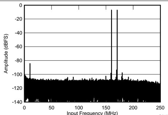
$f_{\text{IN1}} = 160\text{ MHz}$ ,  $f_{\text{IN2}} = 170\text{ MHz}$ ,  $\text{IMD} = 102.68\text{ dBFS}$ ,
