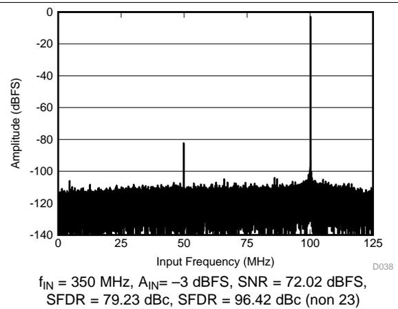
图 39. FFT for 350-MHz Input Signal
