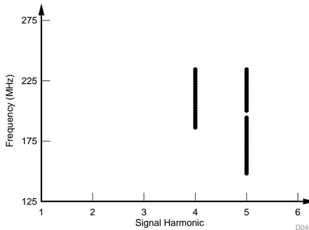
NOTE:  $f_{CLK} = 983.04$  MHz, signal band = 134.32 MHz to 234.32 MHz.
