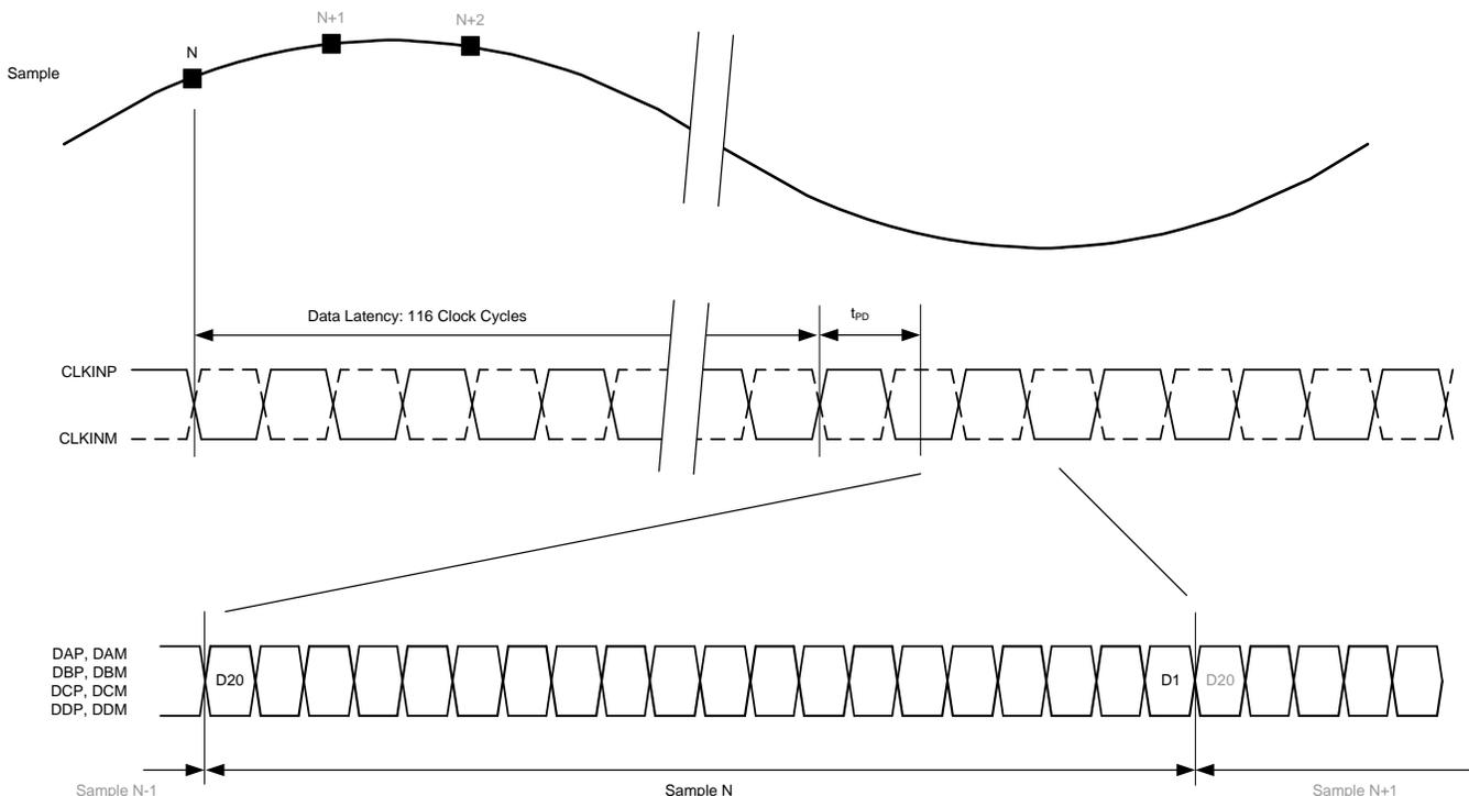
图 1. Latency Timing Diagram in DDC Bypass Mode
