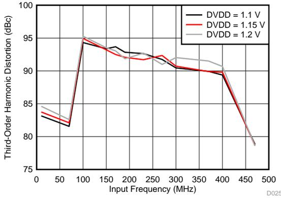
图 26. HD3 vs Input Frequency and DVDD Supply
