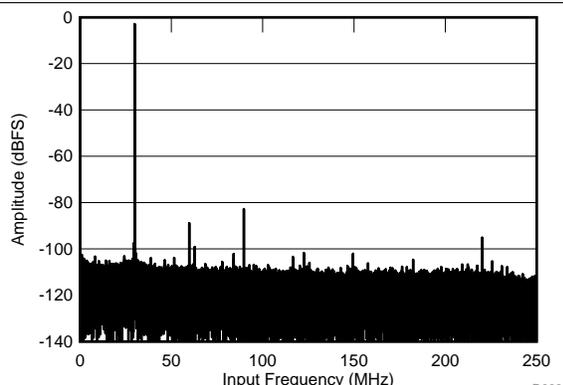
$f_{\text{IN}} = 470\text{ MHz}$ ,  $A_{\text{IN}} = -3\text{ dBFS}$ ,  $\text{SNR} = 68.21\text{ dBFS}$ ,
