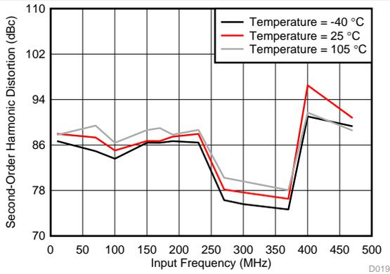
图 20. HD2 vs Input Frequency and Temperature
