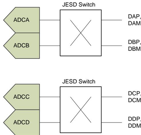
图 68. Switching the Output Lanes
