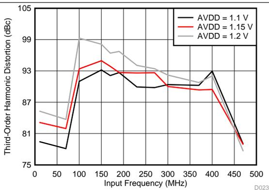
图 24. HD3 vs Input Frequency and AVDD Supply
