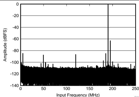
$f_{\text{IN}} = 190\text{ MHz}$ ,  $A_{\text{IN}} = -1\text{ dBFS}$ ,  $f_{\text{Noise}} = 5\text{ MHz}$ ,  $A_{\text{Noise}} = 50\text{ mV}_{\text{PP}}$ , SFDR = 63.12 dBFS
