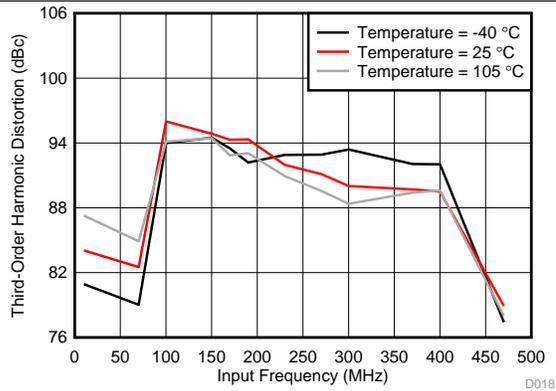
图 19. HD3 vs Input Frequency and Temperature
