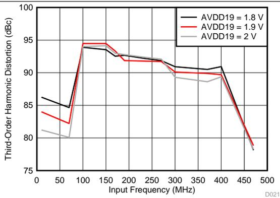
图 22. HD3 vs Input Frequency and AVDD19 Supply
