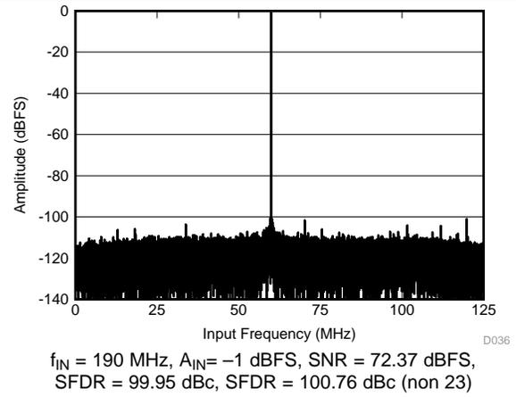
图 37. FFT for 190-MHz Input Signal
