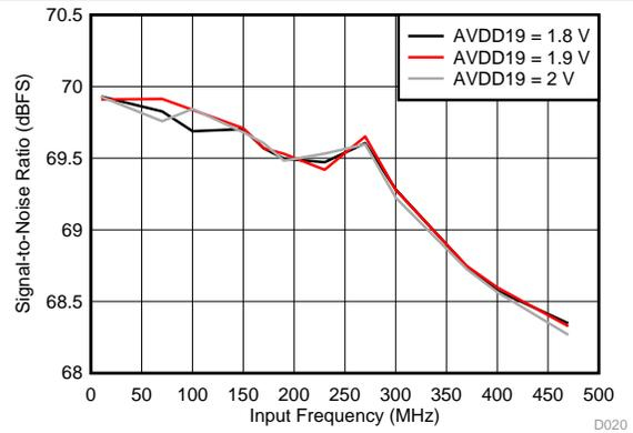
图 21. SNR vs Input Frequency and AVDD19 Supply
