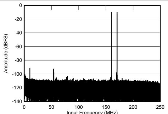
$f_{\text{IN1}} = 160\text{ MHz}$ ,  $f_{\text{IN2}} = 170\text{ MHz}$ ,  $\text{IMD} = 103.44\text{ dBFS}$ ,
