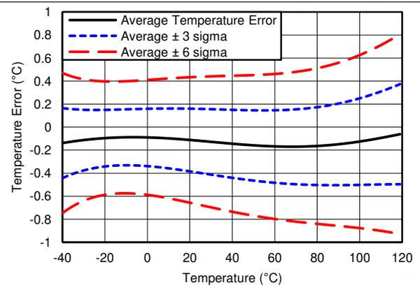
Figure 7. Temperature Sensor Error vs Temperature
