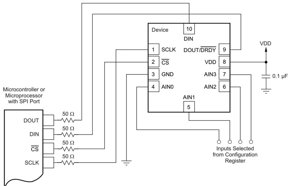
**Figure 18. Typical Connections**
