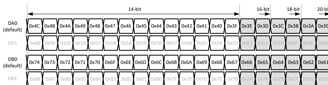
图 8-38. 1-wire output bit mapping
