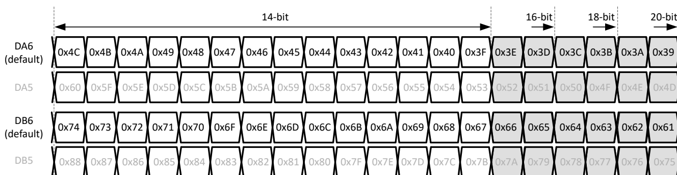
图 8-40. 1-wire output bit mapping
