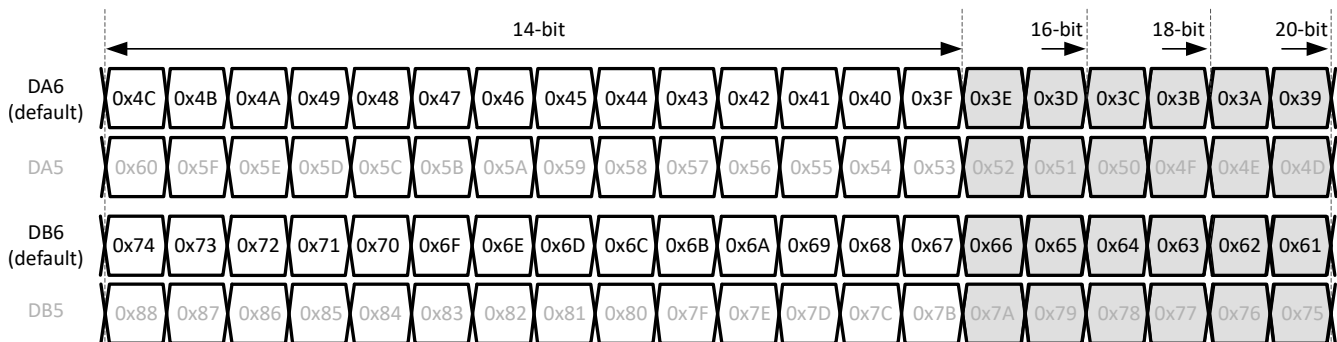
图 8-46. 1-wire output bit mapping
