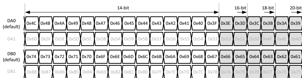
图 8-45. 1-wire output bit mapping
