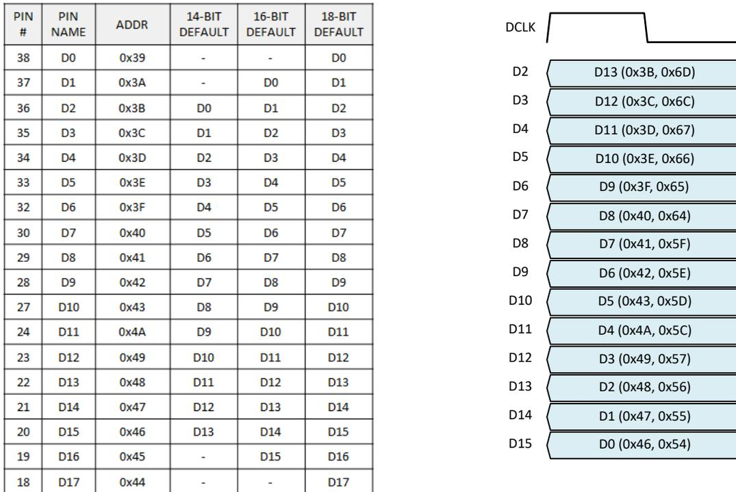
**图 8-43. SDR output mapping (left) and example (right)**
