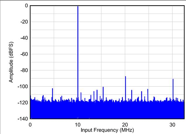
图 6-40. Single Tone FFT at  $F_{IN} = 10\text{ MHz}$
