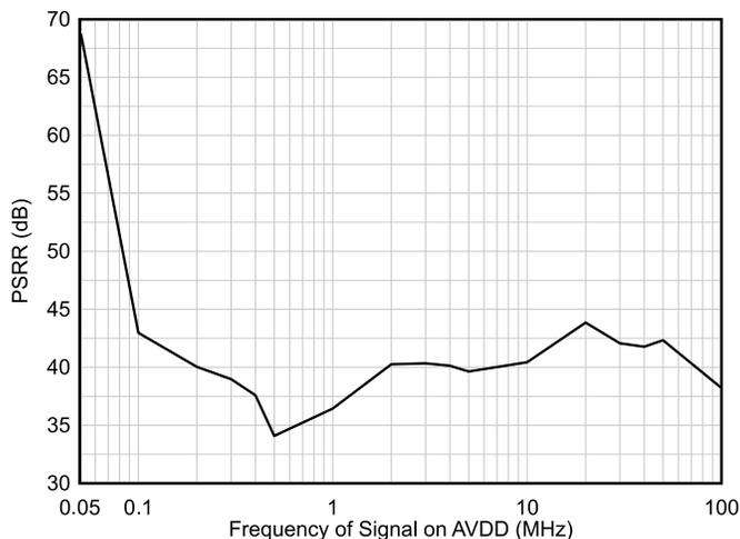
**图 10-1. Power supply rejection ratio (PSRR) vs frequency**
