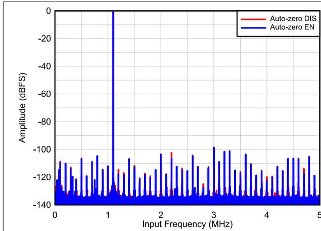
图 8-9.  $F_S = 10 \text{ MSPS}$ ,  $F_{IN} = 1.1 \text{ MHz}$
