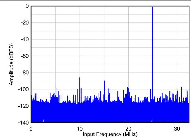
图 6-42. Single Tone FFT at  $F_{IN} = 40\text{ MHz}$
