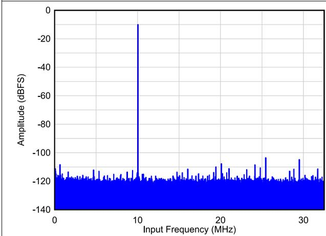
图 6-41. Single Tone FFT at  $F_{IN} = 10\text{ MHz}$
