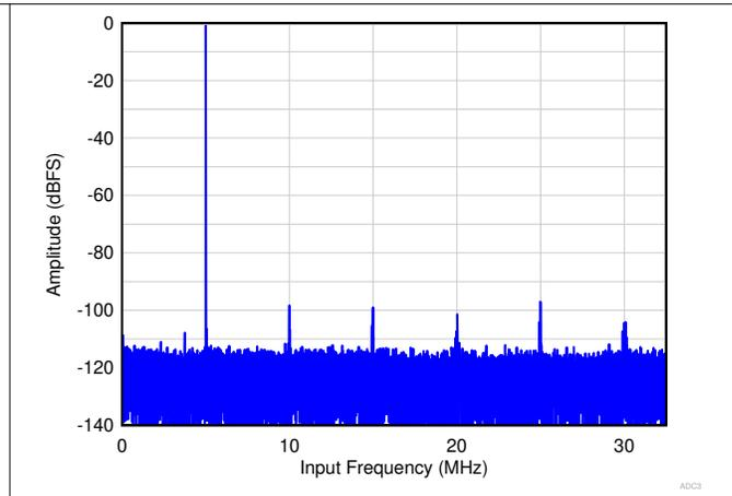
图 9-3. Single Tone FFT at  $F_{IN} = 5$  MHz
