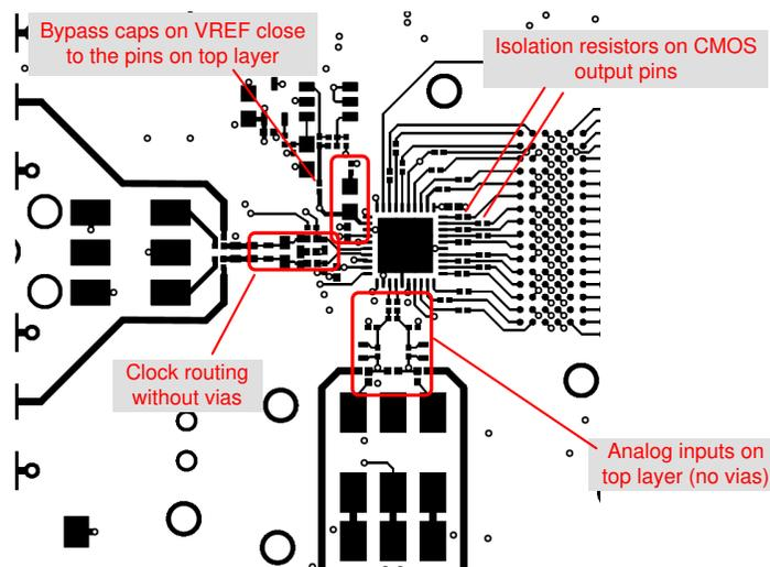
图 11-1. Layout example: top layer of ADC354x EVM
