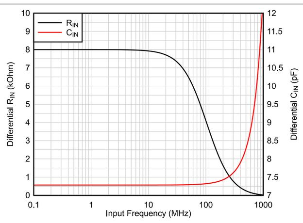
图 8-3. Equivalent  $R_{IN}$ ,  $C_{IN}$  vs Input Frequency
