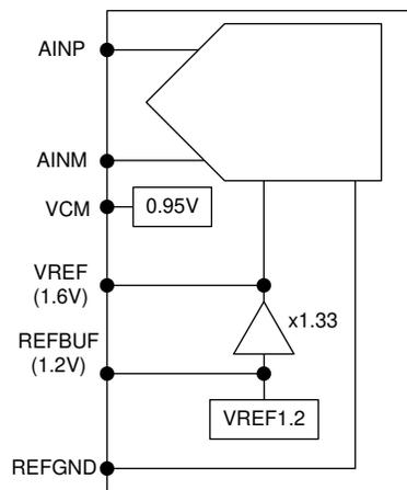
**图 8-16. Different voltage reference options for ADC354x**
