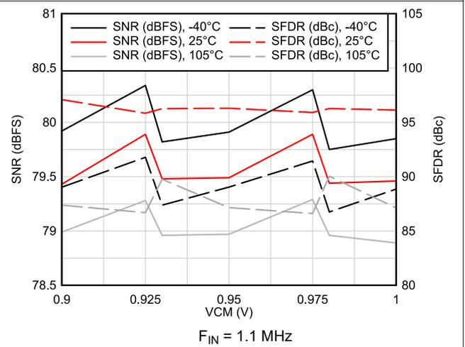
图 6-10. AC Performance vs VCM vs Temperature
