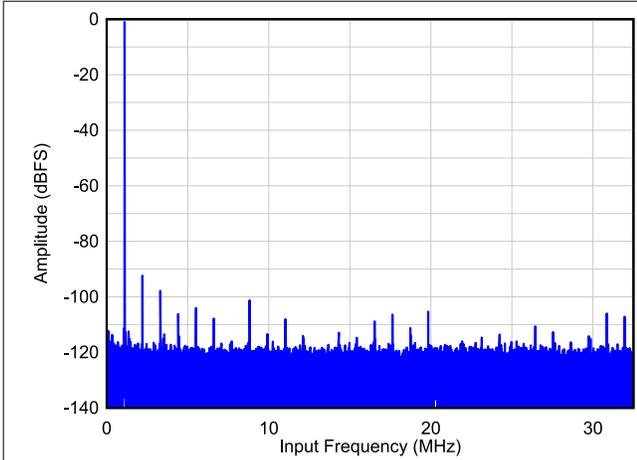
图 6-39. Single Tone FFT at  $F_{IN} = 1.1\text{ MHz}$
