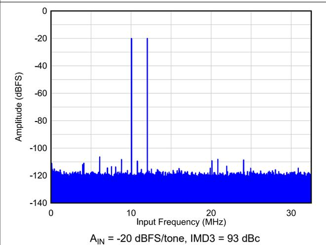
图 6-46. Two Tone FFT at  $F_{IN} = 10, 12$  MHz
