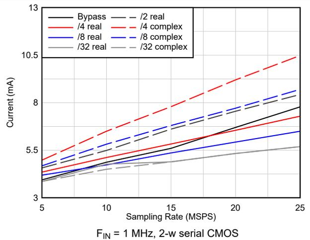
图 6-16. I<sub>OVDD</sub> Current vs Decimation
