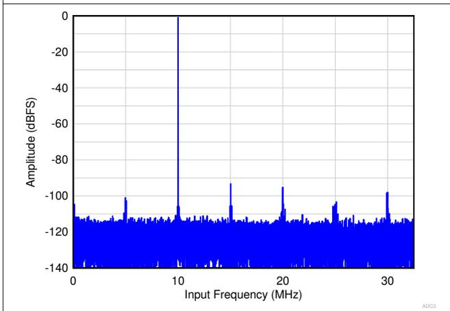
图 9-4. Single Tone FFT at  $F_{IN} = 10$  MHz
