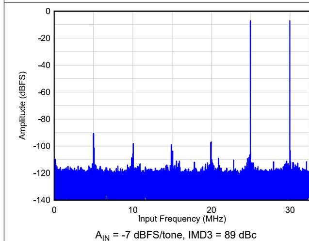
图 6-47. Two Tone FFT at  $F_{IN} = 35, 40$  MHz
