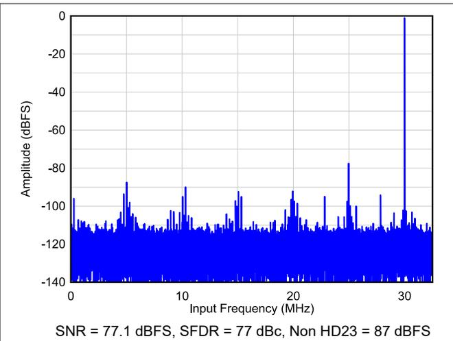
图 6-44. Single Tone FFT at  $F_{IN} = 100$  MHz
