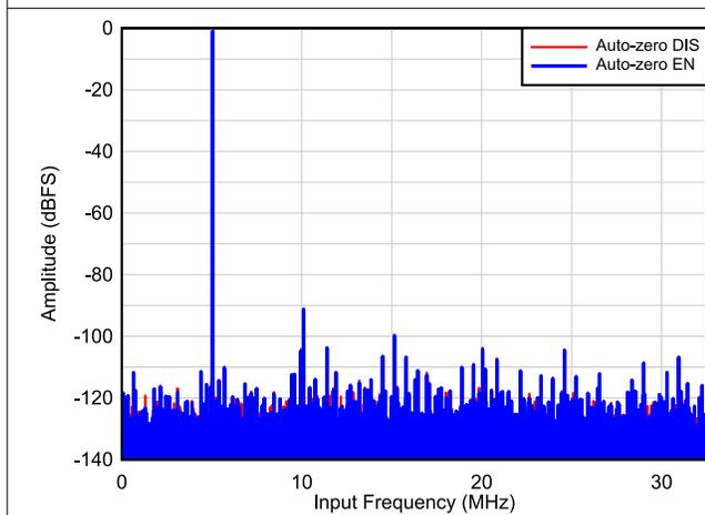
图 8-13.  $F_S = 65 \text{ MSPS}$ ,  $F_{IN} = 5 \text{ MHz}$
