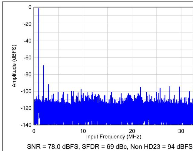
图 6-43. Single Tone FFT at  $F_{IN} = 64$  MHz
