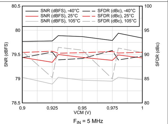
图 6-54. AC Performance vs VCM vs Temperature
