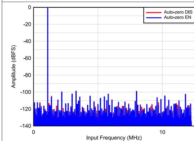
图 8-11.  $F_S = 25 \text{ MSPS}$ ,  $F_{IN} = 1.1 \text{ MHz}$
