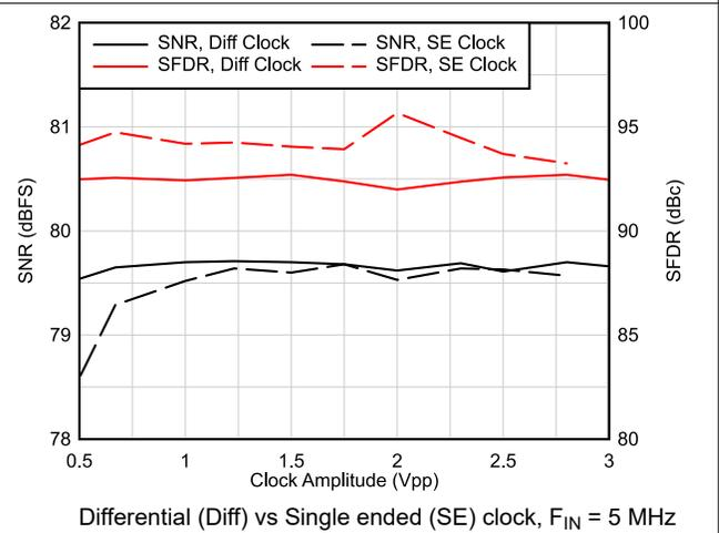
Differential (Diff) vs Single ended (SE) clock, F<sub>IN</sub> = 5 MHz
