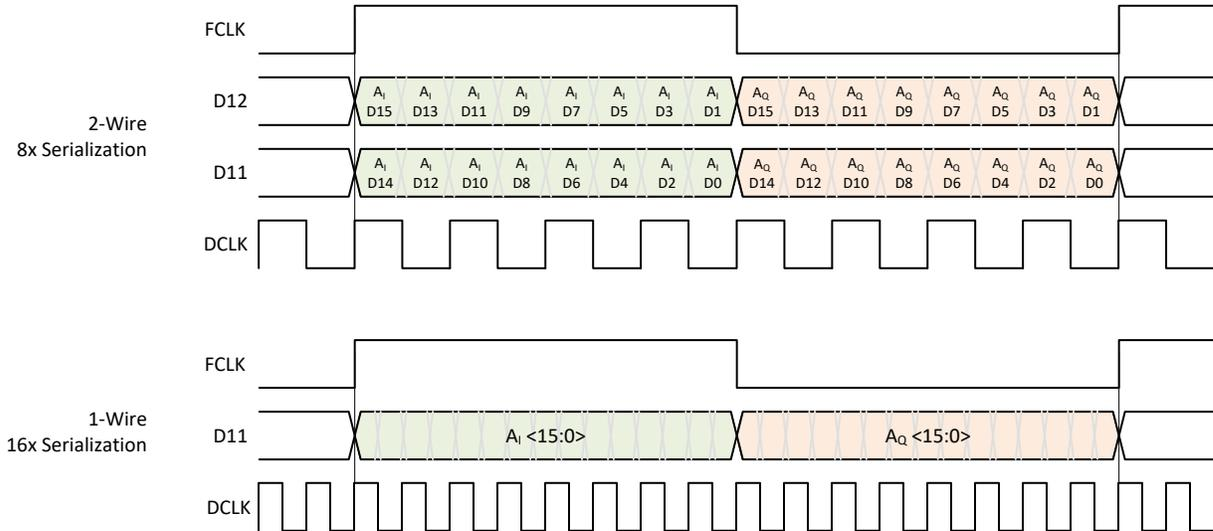
图 8-38. Output Data Format in Complex Decimation
