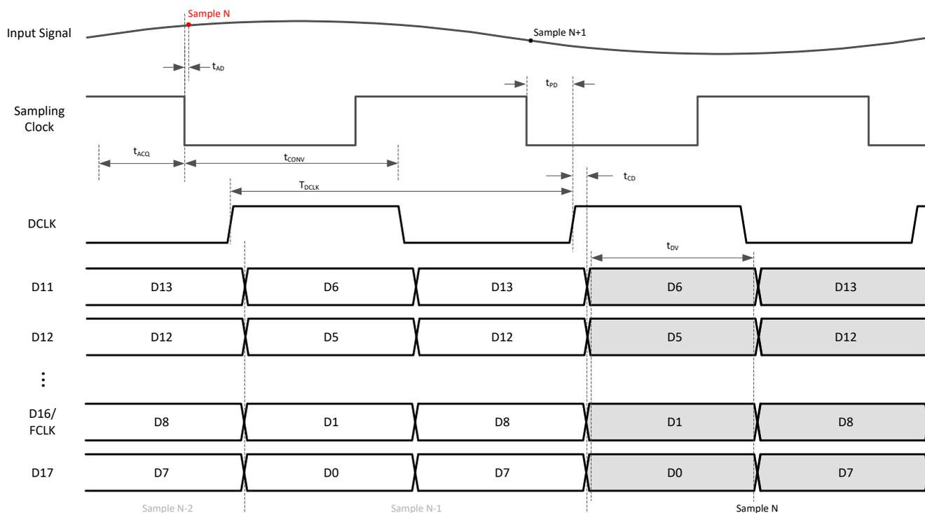
图 7-2. Timing Diagram: DDR CMOS (default bit mapper)
