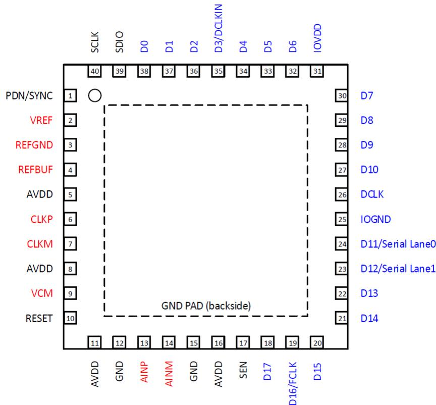
图 5-1. RSB Package, 40-Pin WQFN (Top View)
