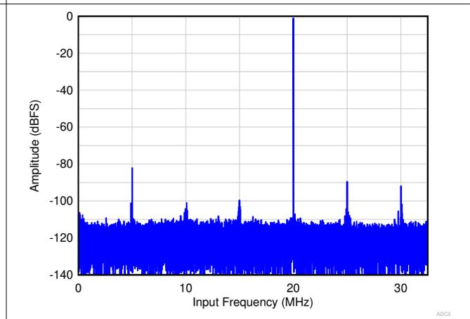
图 9-5. Single Tone FFT at  $F_{IN} = 20$  MHz
