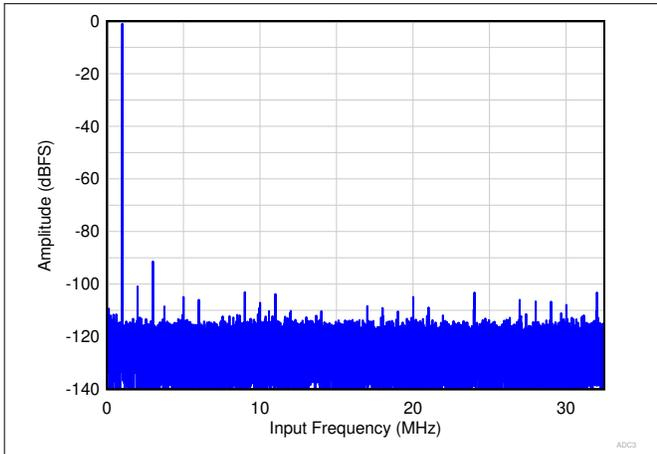
图 9-2. Single Tone FFT at  $F_{IN} = 1$  MHz
