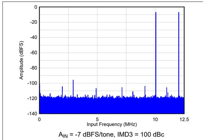
图 6-24. Two Tone FFT at  $F_{IN} = 10, 12$  MHz
