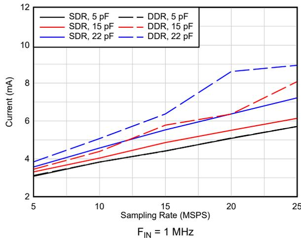
图 6-17. I<sub>OVDD</sub> Current vs Output Load
