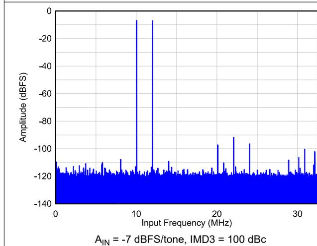
图 6-45. Two Tone FFT at  $F_{IN} = 10, 12$  MHz
