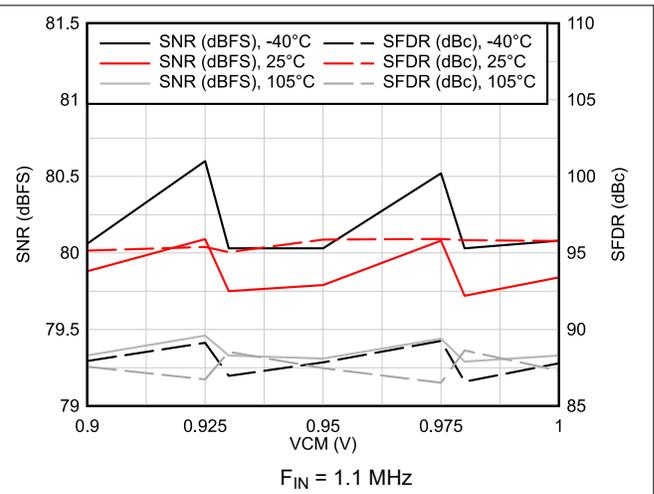
图 6-31. AC Performance vs VCM vs Temperature
