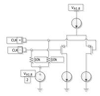
Figure 25. Equivalent Clock Receiver
