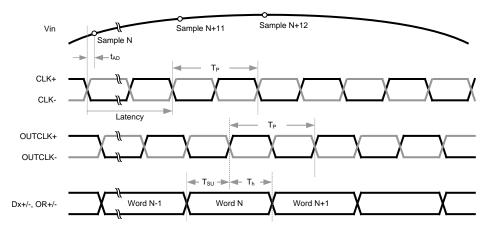
Figure 2. Digital Output Timing
