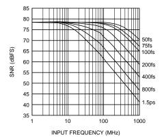
Figure 28. SNR with given Jitter vs. Input Frequency
