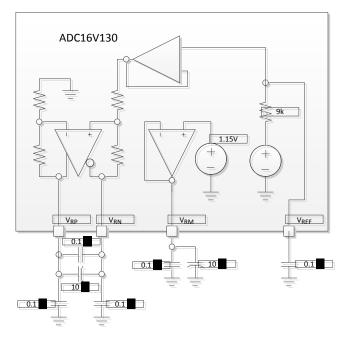
Figure 29. Internal References and their Decoupling
