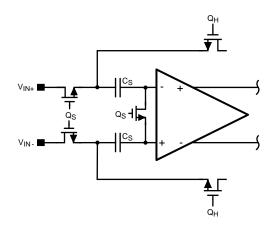
Figure 20. Simplified Switched-Capacitor Sample-and-hold Circuit
