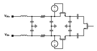
Figure 23. Input Equivalent Circuit
