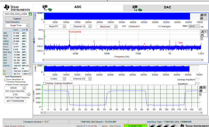
图 8-11. 200-MHz, Sine-Wave (Channel A) Frequency Domain (FFT) and 40-MHz, Square-Wave (Channel B) Time Domain for 5-GSPS, Single-Channel Oscilloscope
