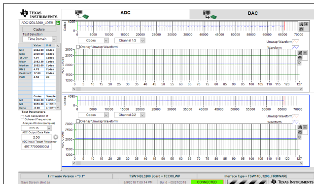
图 8-9. Idle-Channel Noise (No Input) for 2.5-GSPS, Dual-Channel Oscilloscope
