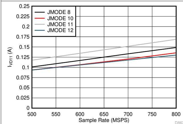
图 5-109. Single Channel,  $I_{VD11}$  vs  $F_S$  for JMODES 8 - 12
