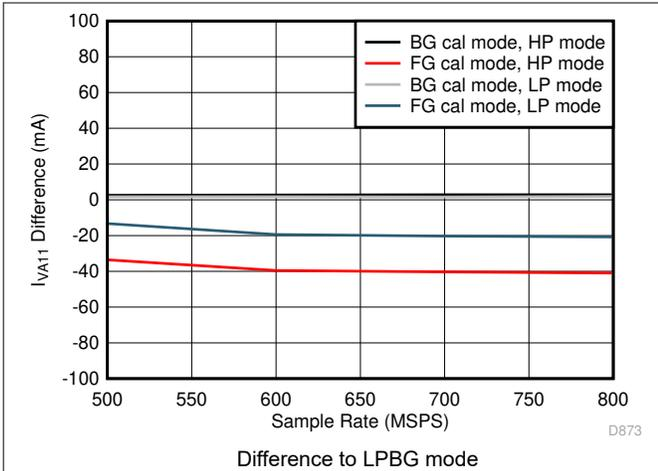
图 5-113. Single Channel,  $I_{VA11}$  vs  $F_S$  over Modes
