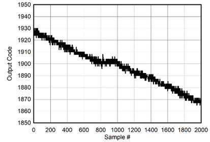
BG Calibration, midscale input voltage, ADC\_SRC\_DLY=31,
