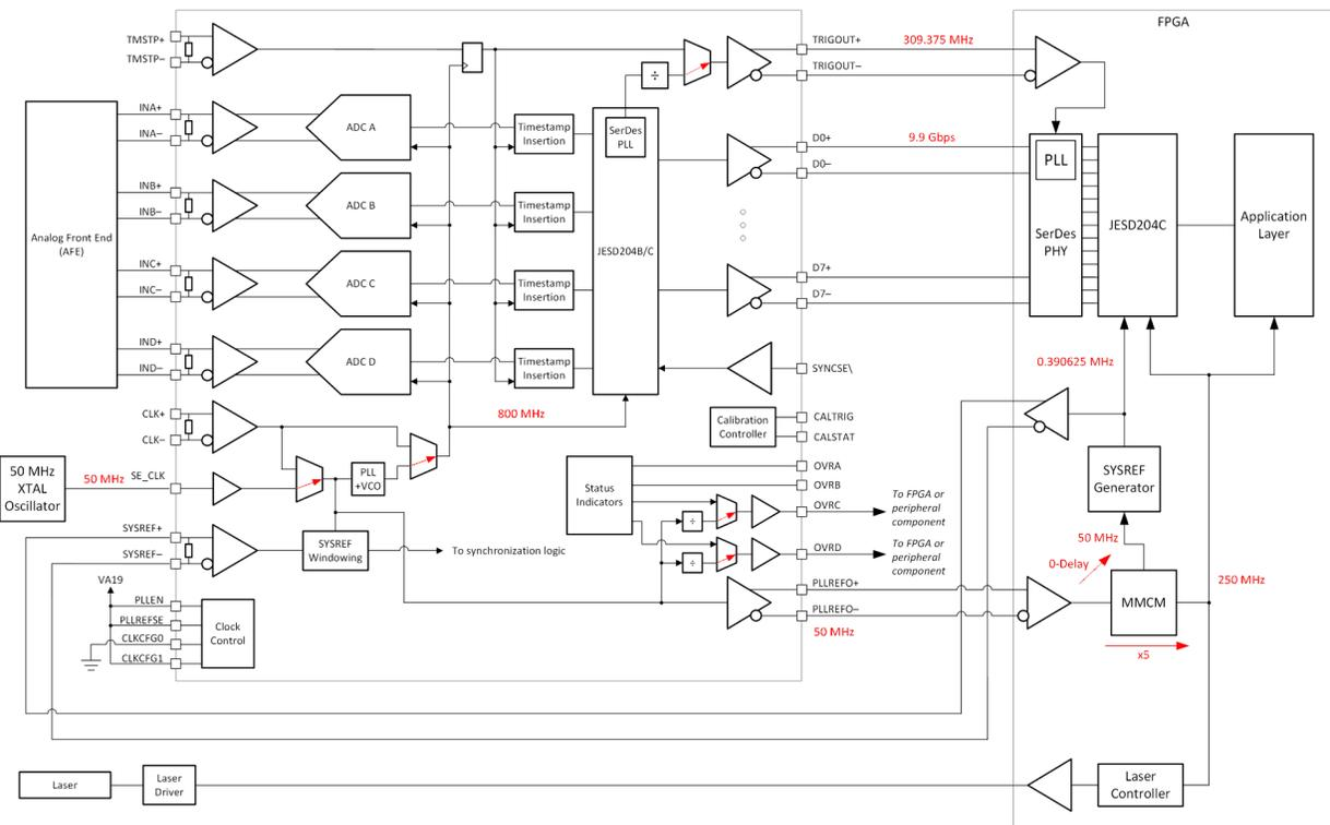
图 7-1. Typical Configuration for a LiDAR Digitizer
