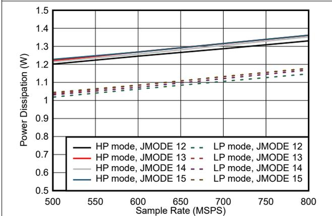
图 5-91. Dual Channel, Power Dissipation vs  $F_S$  for JMODES 12 - 15
