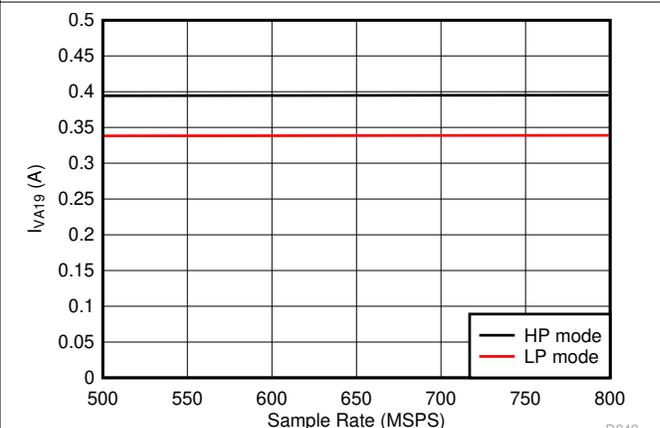
图 5-92. Dual Channel,  $I_{VA19}$  vs  $F_S$
