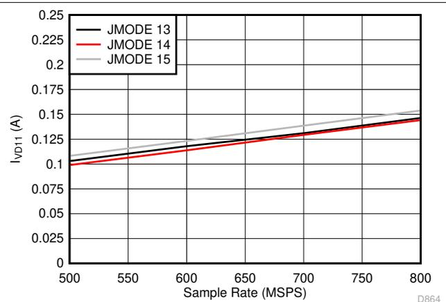
图 5-110. Single Channel,  $I_{VD11}$  vs  $F_S$  for JMODES 13 - 15
