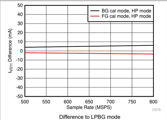
图 5-114. Single Channel,  $I_{VD11}$  vs  $F_S$  over Modes
