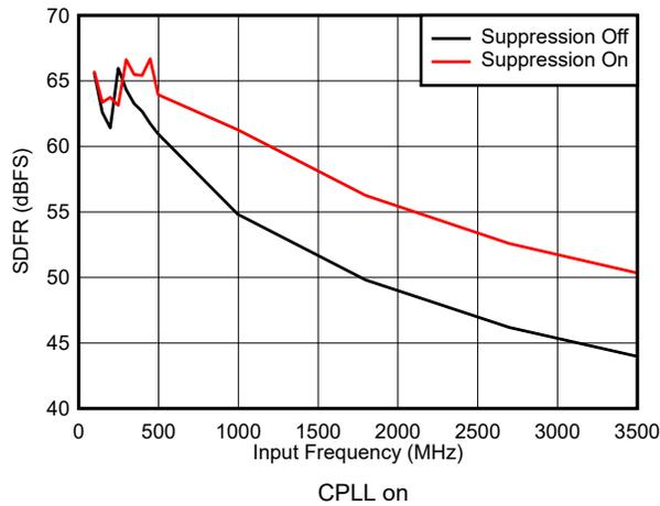
图 5-35. SFDR vs Input Frequency and Suppression
