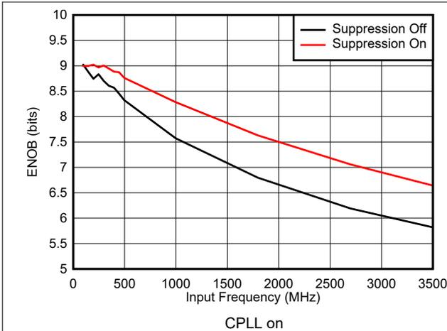
图 5-37. ENOB vs Input Frequency and Suppression
