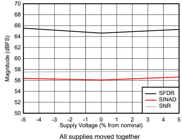
图 5-38. SNR, SFDR and SINAD vs Supply Voltage
