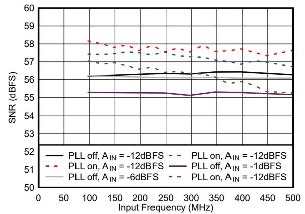
图 5-48. SNR vs Input Frequency in Low Power Mode
