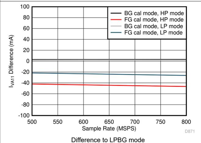
图 5-86. Quad Channel,  $I_{VA11}$  vs  $F_S$  over Modes
