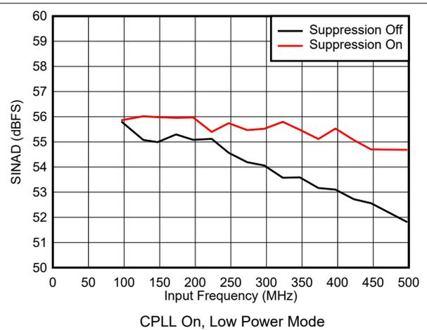
图 5-62. SINAD vs Input Frequency
