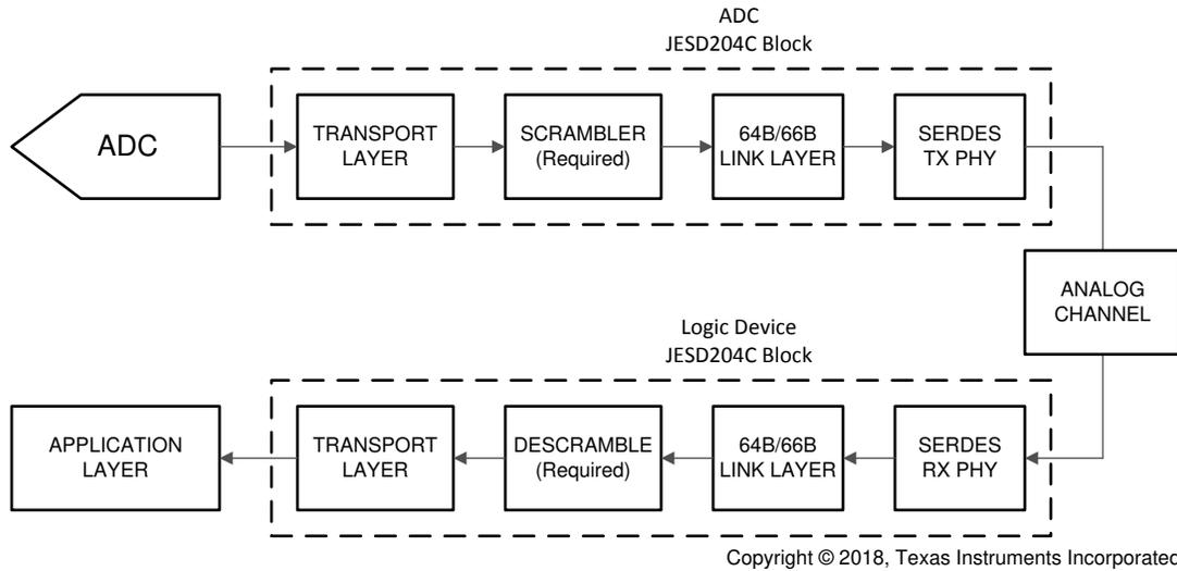
图 6-8. Simplified 64B/66B Encoded JESD204C Interface Diagram
