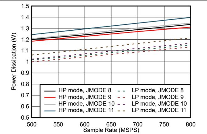
图 5-90. Dual Channel, Power Dissipation vs  $F_S$  for JMODES 8 - 11
