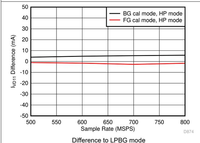
图 5-87. Quad Channel,  $I_{VD11}$  vs  $F_S$  over Modes
