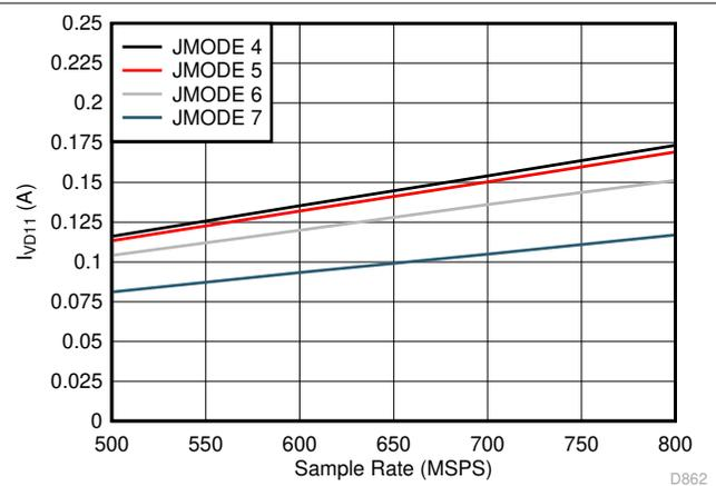
图 5-108. Single Channel,  $I_{VD11}$  vs  $F_S$  for JMODES 4 - 7
