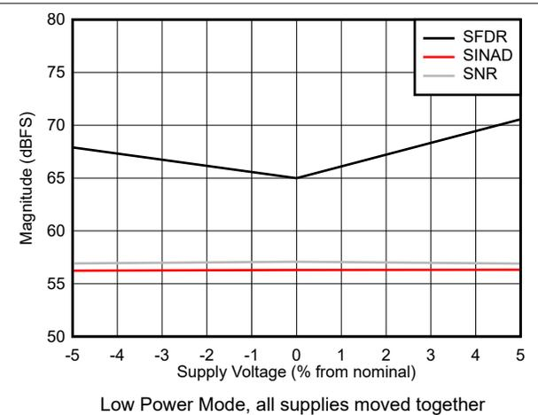
图 5-64. SNR, SFDR and SINAD vs Supply Voltage
