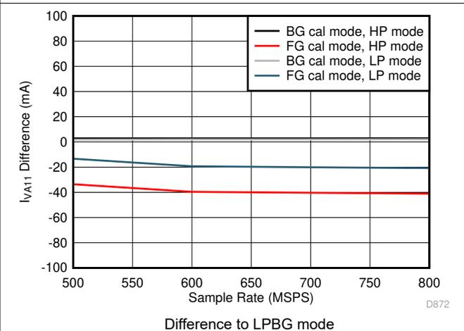
图 5-100. Dual Channel,  $I_{VA11}$  vs  $F_S$  over Modes
