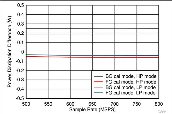
图 5-98. Dual Channel, Power Dissipation vs  $F_S$  over Modes
