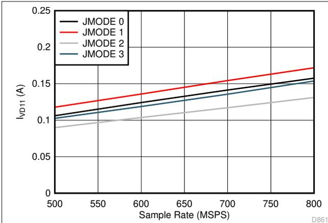
图 5-107. Single Channel,  $I_{VD11}$  vs  $F_S$  for JMODES 0 - 3
