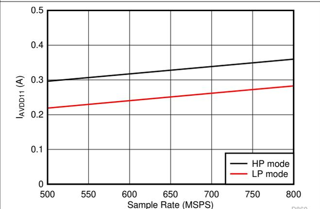
图 5-106. Single Channel,  $I_{VA11}$  vs  $F_S$
