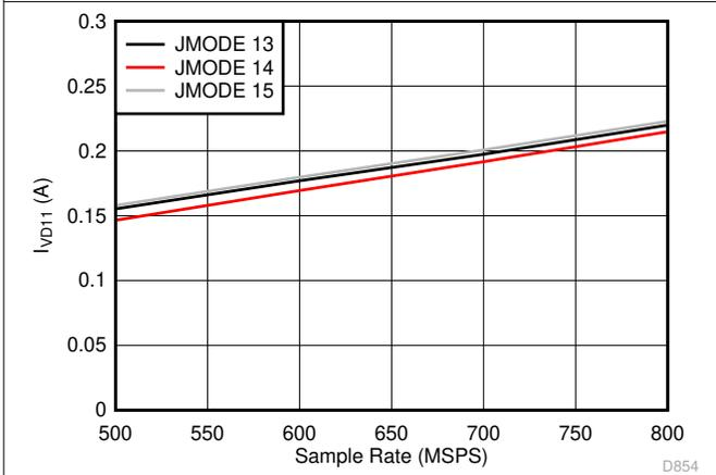
图 5-97. Dual Channel,  $I_{VD11}$  vs  $F_S$  for JMODES 13 - 15
