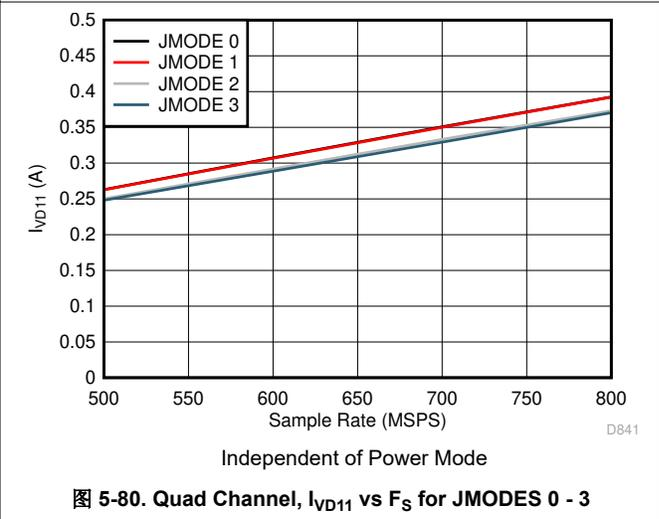
图 5-80. Quad Channel,  $I_{VD11}$  vs  $F_S$  for JMODES 0 - 3
