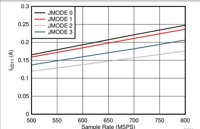
图 5-94. Dual Channel,  $I_{VD11}$  vs  $F_S$  for JMODES 0 - 3
