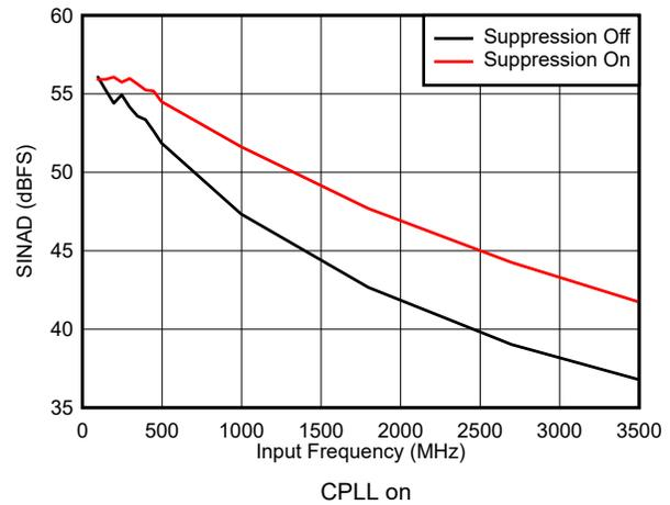
图 5-36. SINAD vs Input Frequency and Suppression
