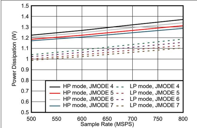
图 5-89. Dual Channel, Power Dissipation vs  $F_S$  for JMODES 4 - 7
