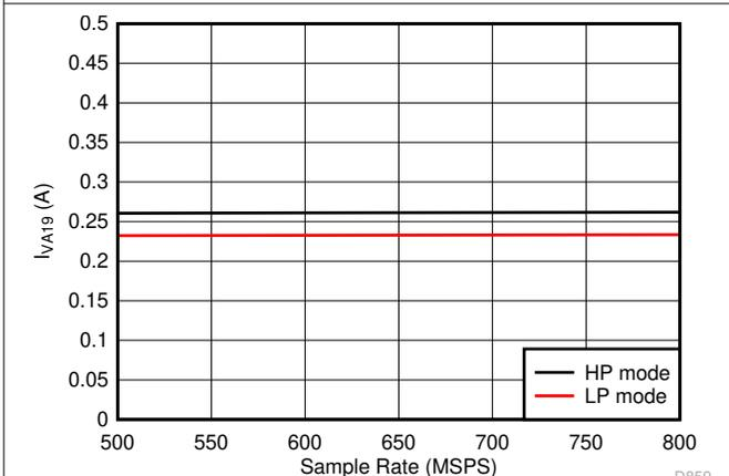
图 5-105. Single Channel,  $I_{VA19}$  vs  $F_S$
