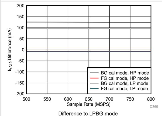
图 5-99. Dual Channel,  $I_{VA19}$  vs  $F_S$  over Modes
