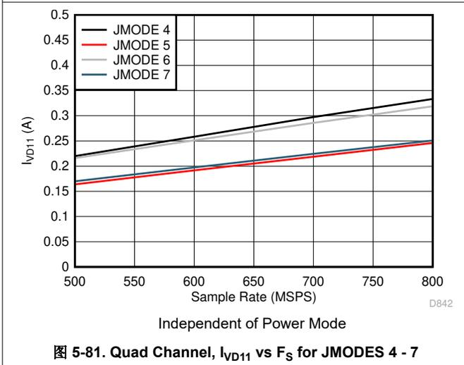
图 5-81. Quad Channel,  $I_{VD11}$  vs  $F_S$  for JMODES 4 - 7
