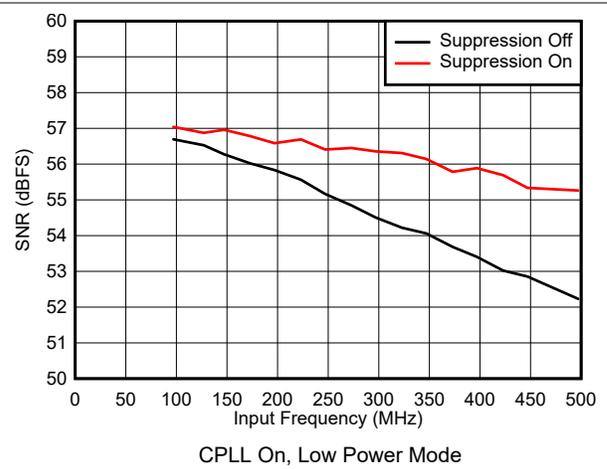
图 5-60. SNR vs Input Frequency
