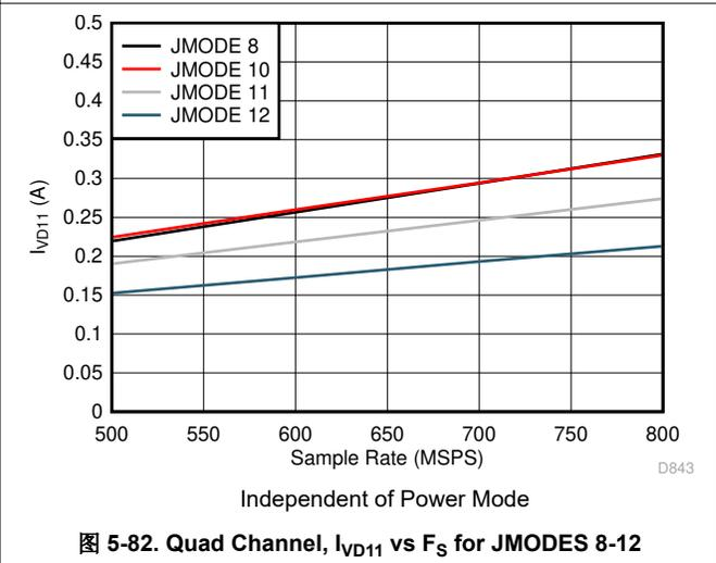
图 5-82. Quad Channel,  $I_{VD11}$  vs  $F_S$  for JMODES 8-12
