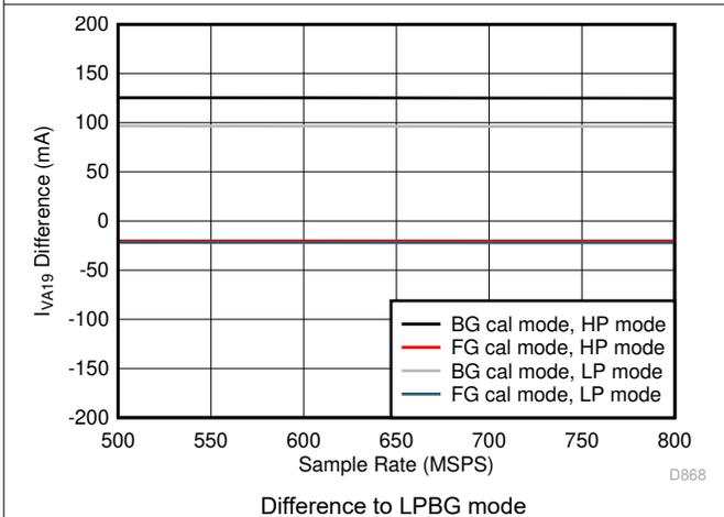
图 5-85. Quad Channel,  $I_{VA19}$  vs  $F_S$  over Modes
