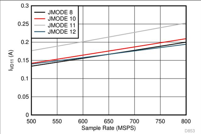
图 5-96. Dual Channel,  $I_{VD11}$  vs  $F_S$  for JMODES 8 - 12
