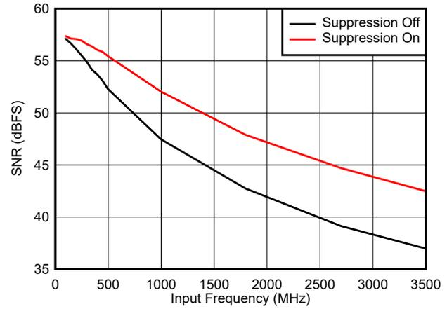
图 5-34. SNR vs Input Frequency and Suppression
