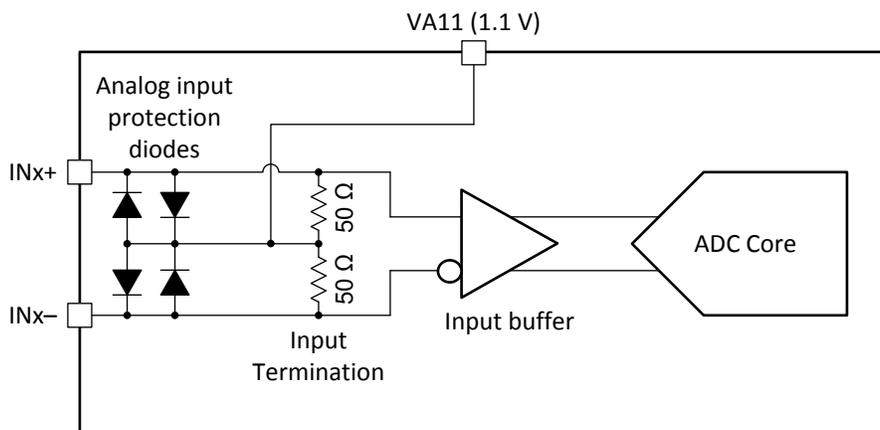
图 6-4. Analog Input Internal Termination and Protection Diagram
