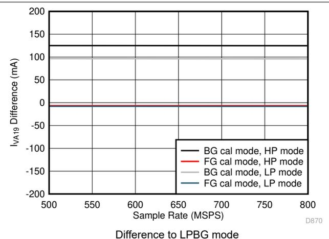
图 5-112. Single Channel,  $I_{VA19}$  vs  $F_S$  over Modes
