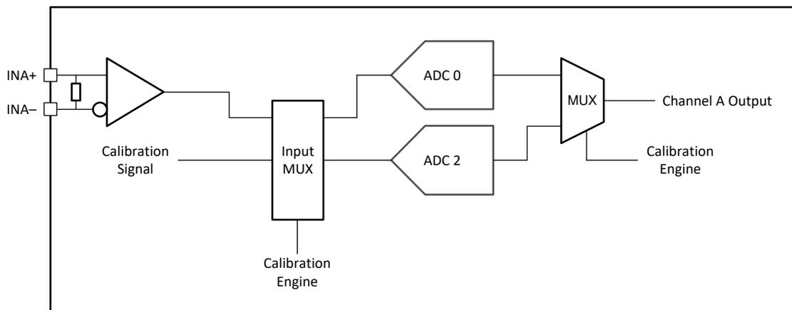
图 6-17. Single Channel Calibration System Block Diagram
