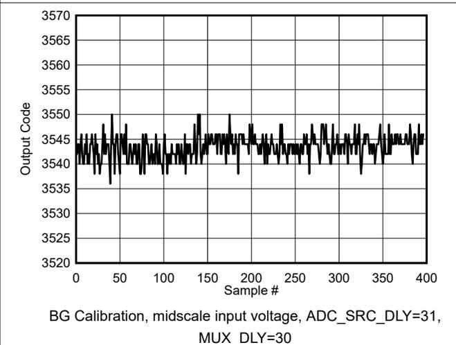
图 5-116. Background Calibration Core Transition (voltage offset)
