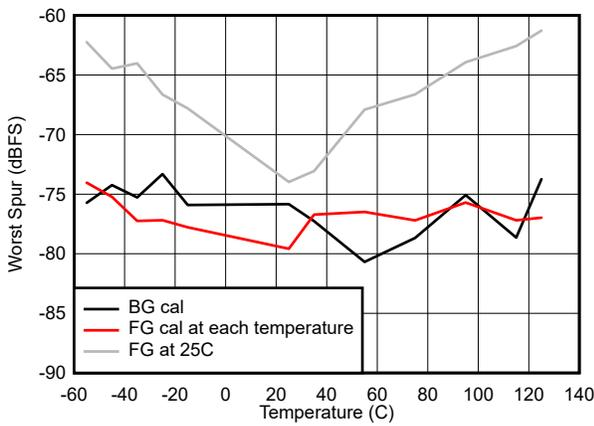
图 5-47. worst non-HD spur vs Temperature
