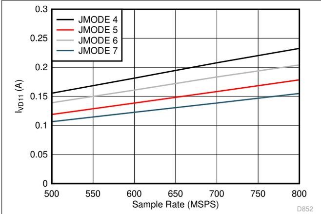
图 5-95. Dual Channel,  $I_{VD11}$  vs  $F_S$  for JMODES 4 - 7
