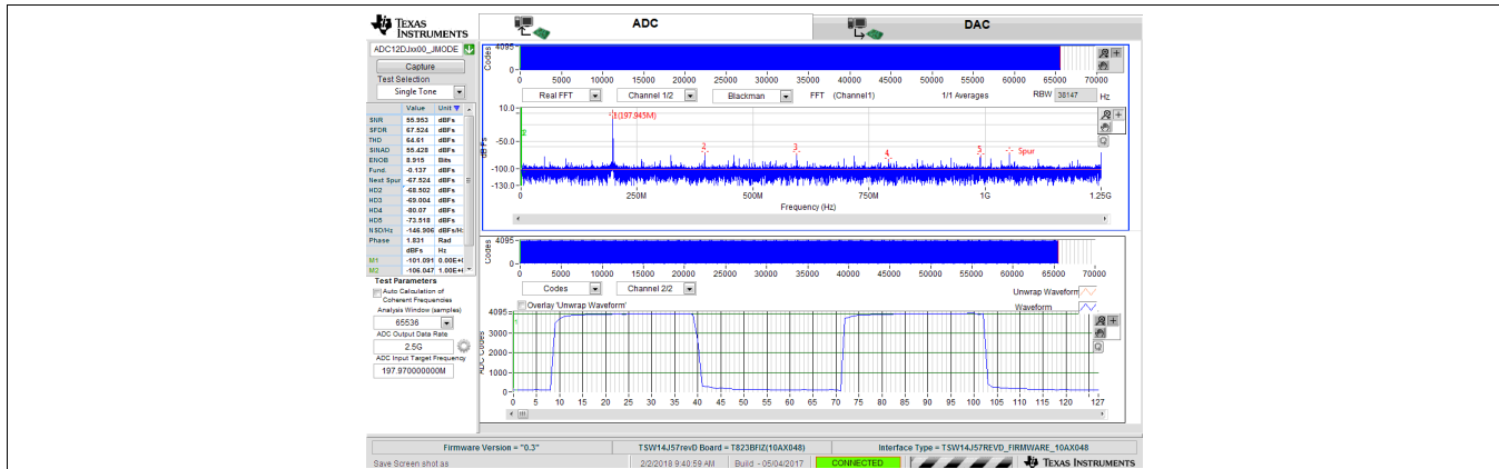
图 191. 200-MHz, Sine-Wave (Channel A) Frequency Domain (FFT) and 40-MHz, Square-Wave (Channel B) Time Domain for 5-GSPS, Single-Channel Oscilloscope
