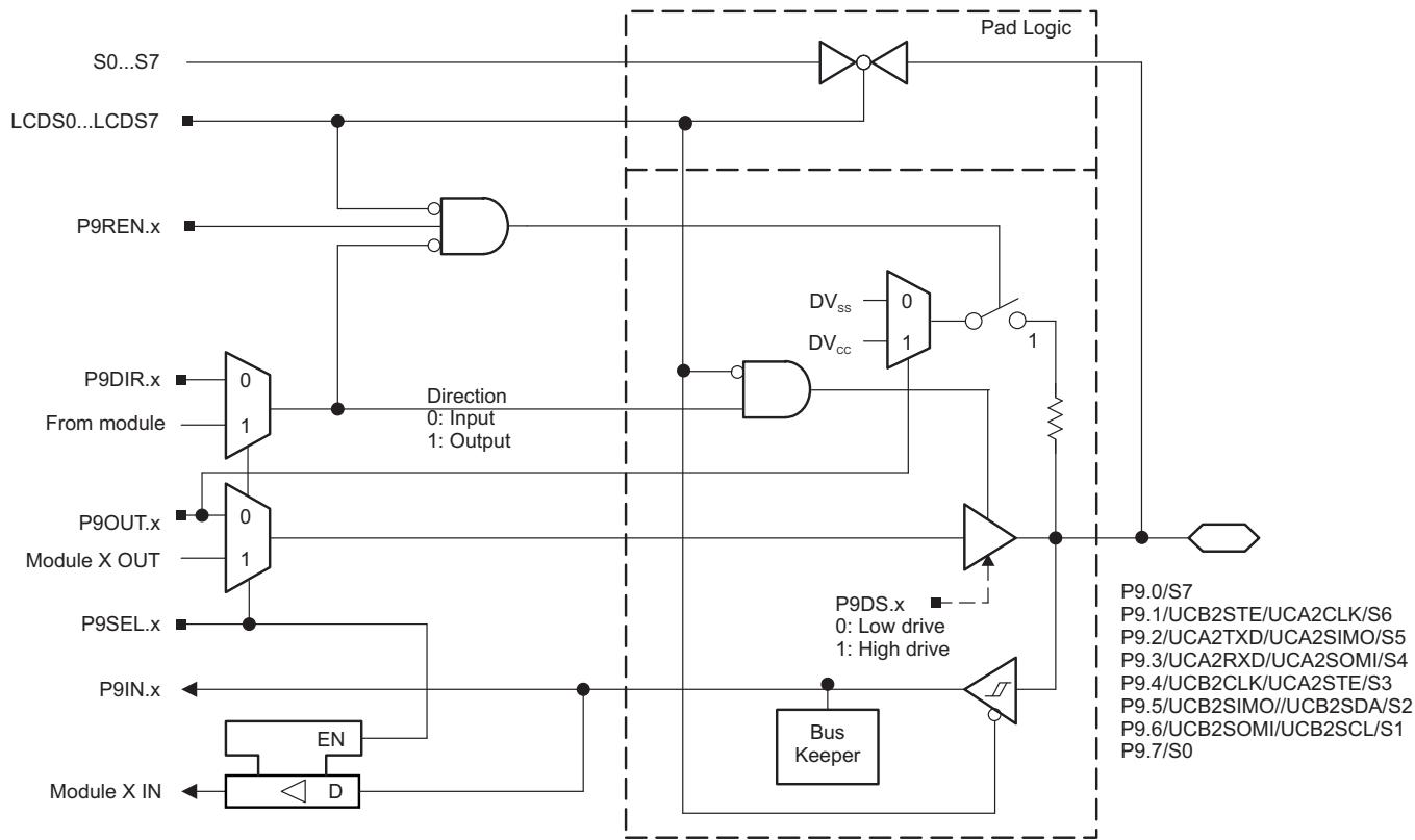
Figure 6-13. Port P9 (P9.0 to P9.7) Schematic
