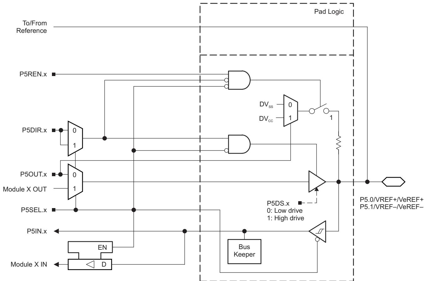
Figure 6-6. Port P5 (P5.0 and P5.1) Schematic
