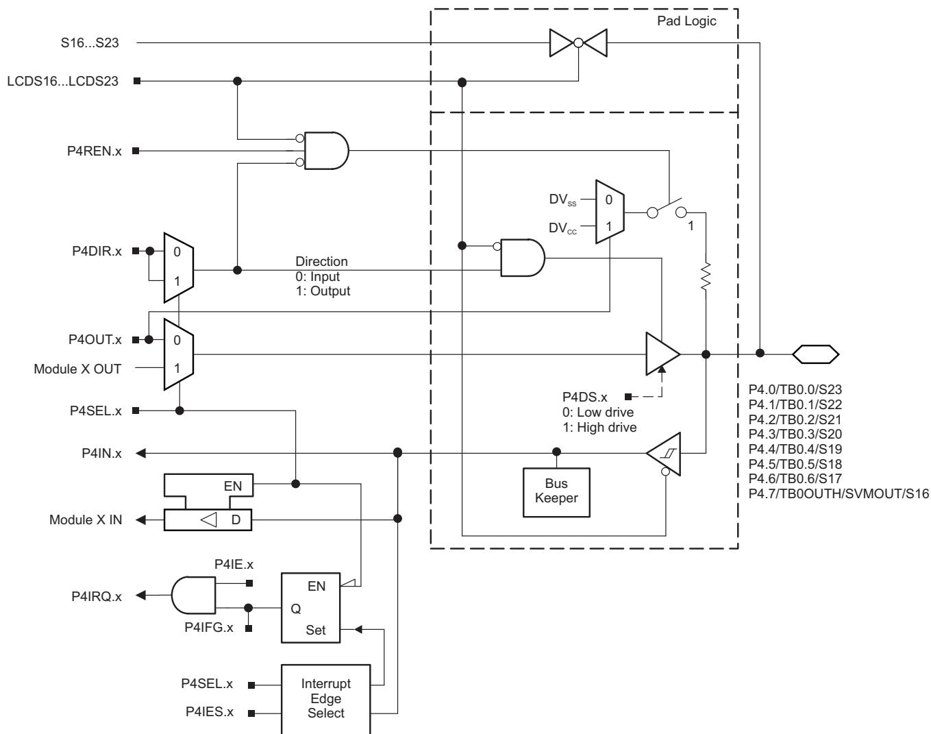
Figure 6-5. Port P4 (P4.0 to P4.7) Schematic
