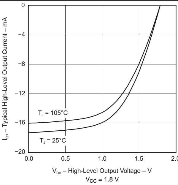
Figure 5-9. Typical High-Level Output Current vs High-Level Output Voltage
