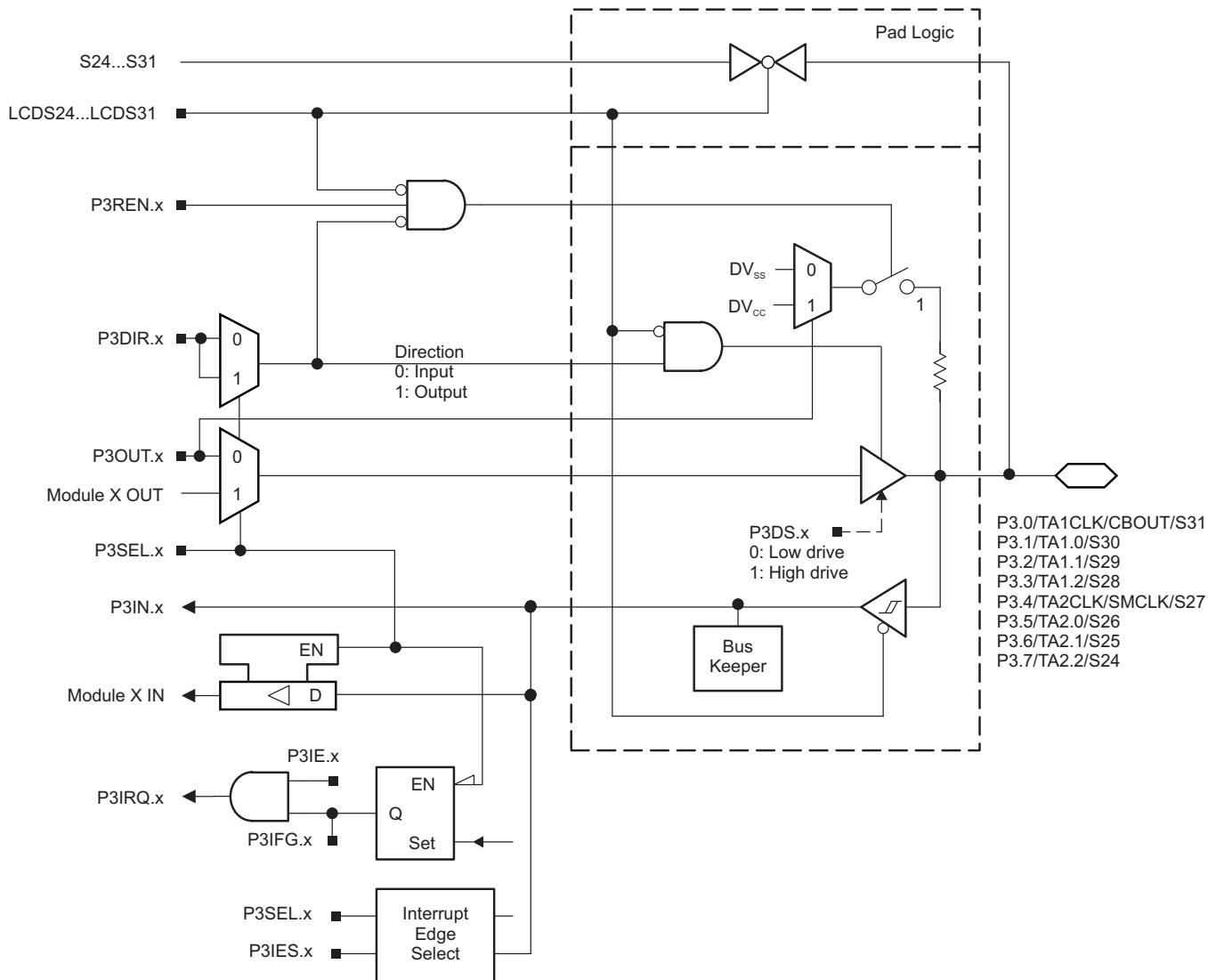
Figure 6-4. Port P3 (P3.0 to P3.7) Schematic
