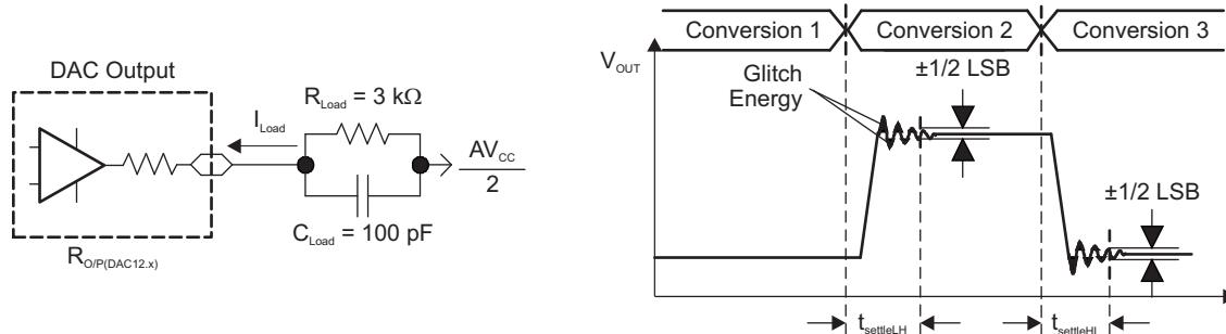
**Figure 5-19. Settling Time and Glitch Energy Testing**
