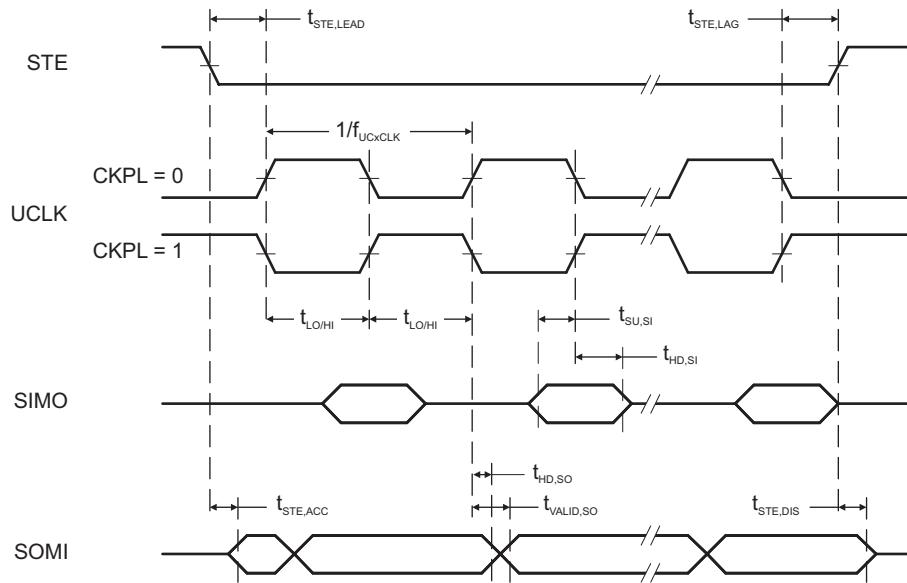
**Figure 5-13. SPI Slave Mode, CKPH = 0**
