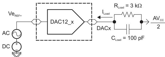
**Figure 5-21. Test Conditions for 3-dB Bandwidth Specification**
