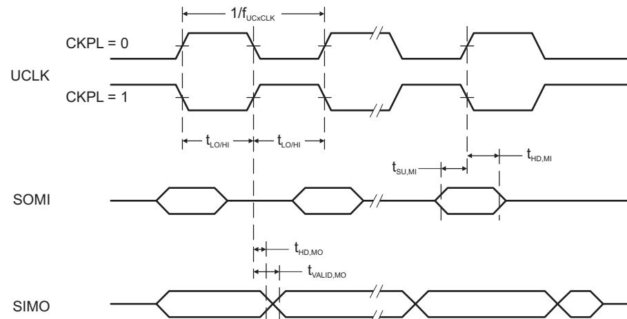
**Figure 5-12. SPI Master Mode, CKPH = 1**
