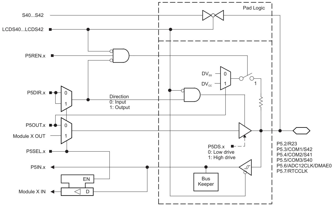
**Figure 6-7. Port P5 (P5.2 to P5.7) Schematic**
