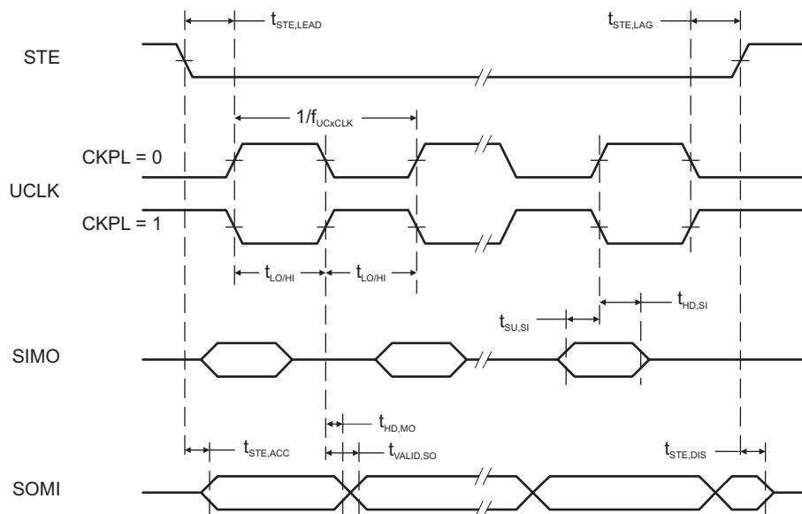
**Figure 5-14. SPI Slave Mode, CKPH = 1**
