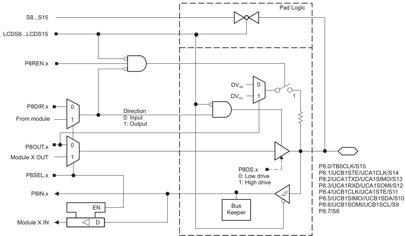
Figure 6-12. Port P8 (P8.0 to P8.7) Schematic
