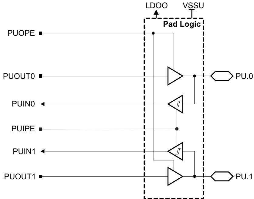
Figure 6-14. Port U (PU.0 and PU.1) Schematic
