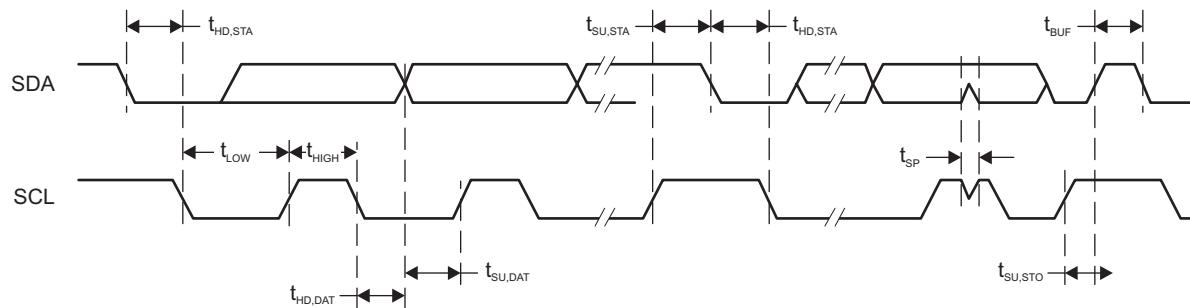
**Figure 5-15. I<sup>2</sup>C Mode Timing**
