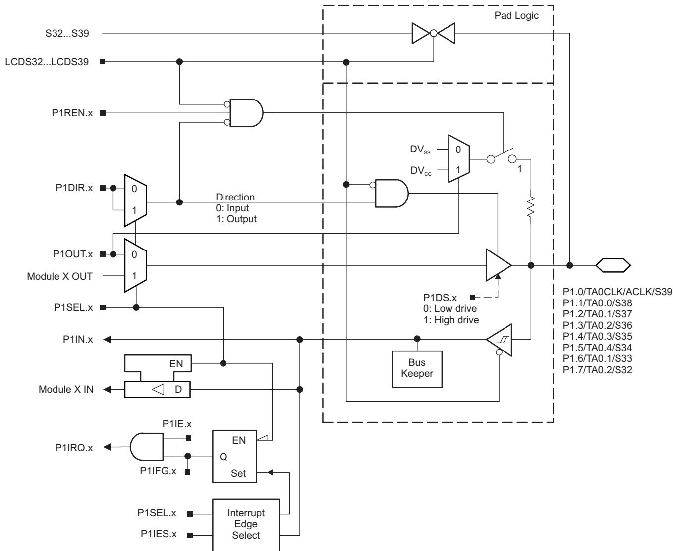
Figure 6-2. Port P1 (P1.0 to P1.7) Schematic
