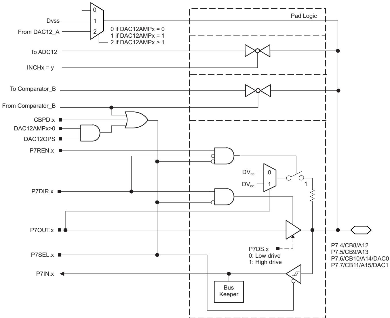
Figure 6-11. Port P7 (P7.4 to P7.7) Schematic
