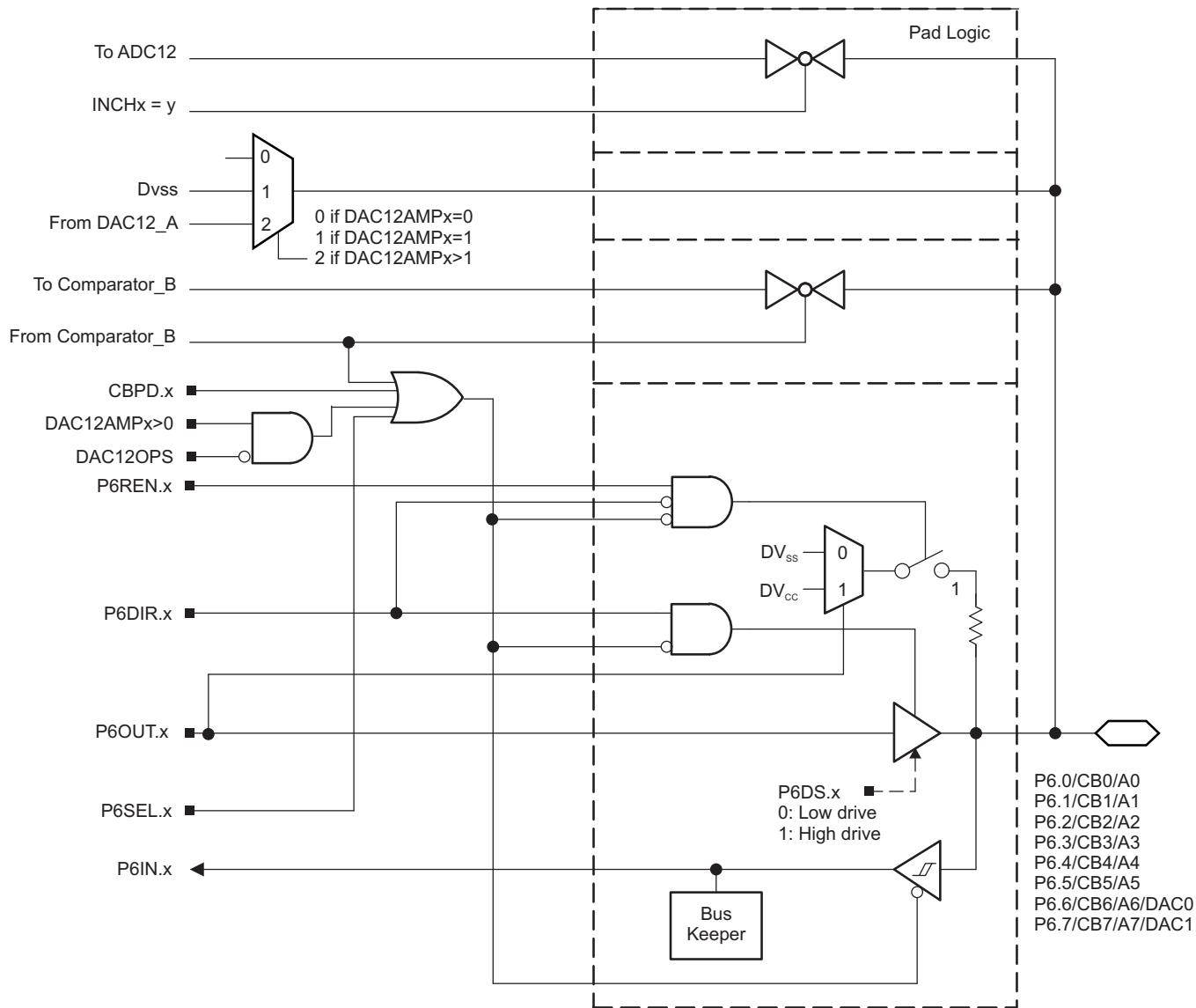
Figure 6-8. Port P6 (P6.0 to P6.7) Schematic
