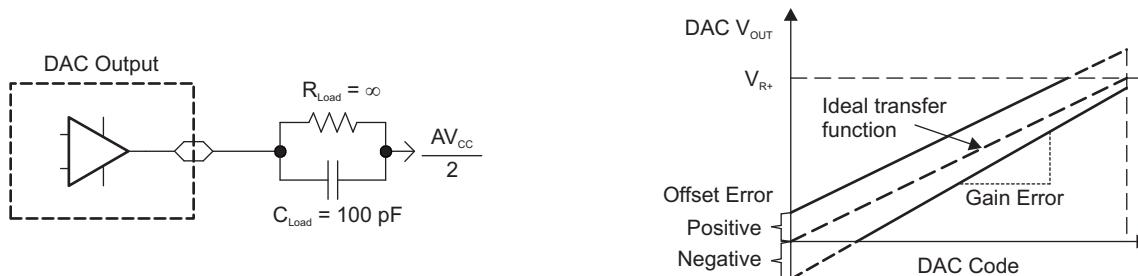
**Figure 5-17. Linearity Test Load Conditions and Gain/Offset Definition**
