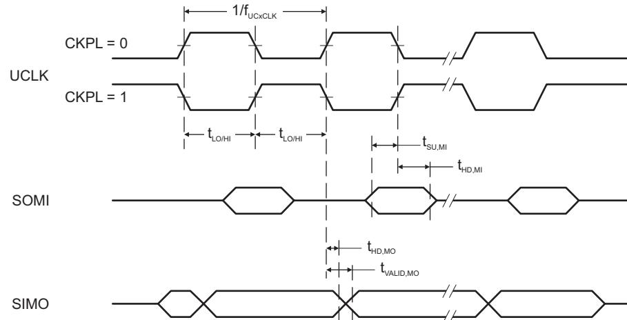
**Figure 5-11. SPI Master Mode, CKPH = 0**
