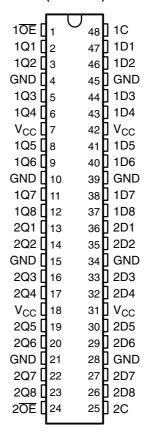
A buffered output-enable (OE) input can be used to place the outputs in either a normal logic state (high or low logic levels) or the high-impedance state. In the high-impedance state, the outputs neither load nor drive the bus lines significantly. The high-impedance state and the increased drive provide the capability to drive bus lines in a bus-organized system without need for interface or pullup components.
